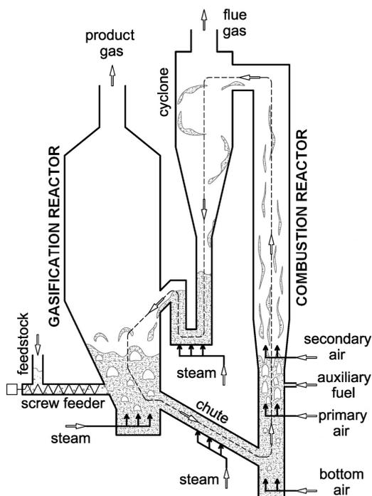
**Figure 2:** Classical dual fluidized bed steam gasifier
