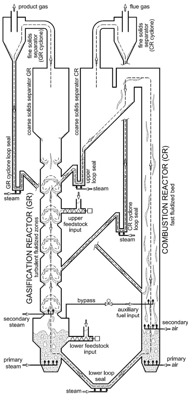
**Figure 4:** G-volution gasification system, next generation biomass gasifier
