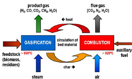
**Figure 1:** Principle of dual fluidized bed steam gasification for solid feedstock (conventional process)
