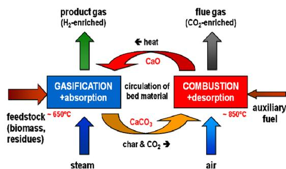
**Figure 3:** Principle of dual fluidized bed steam gasification with selective transport of CO<sub>2</sub> (SERP)
