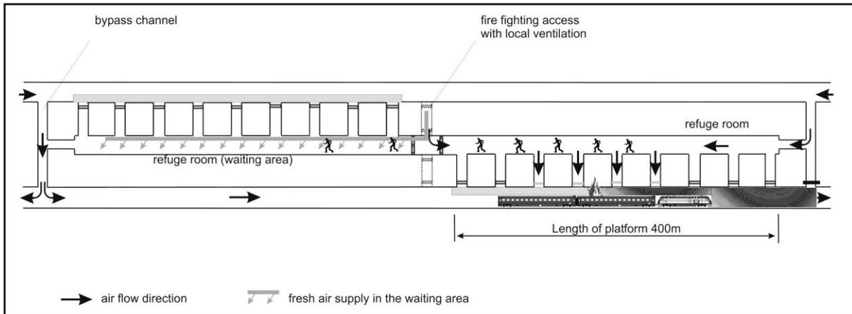
Figure 6: Air flow direction in case of self-rescue (open doors at the escape passages) in the emergency station
