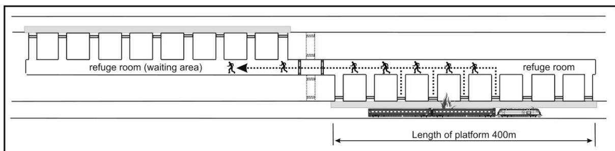
Figure 3: Layout of emergency station
