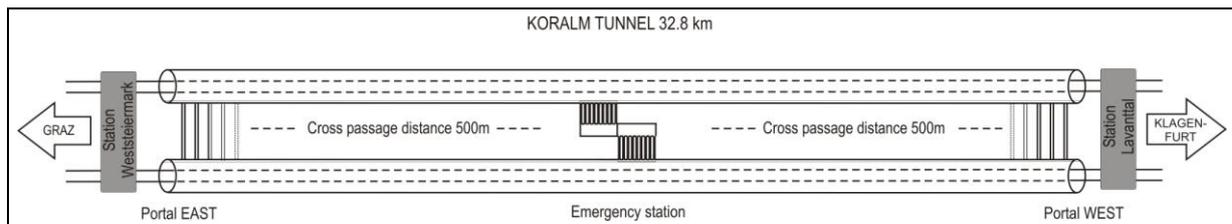
Figure 2: Tunnel system Koralm tunnel
