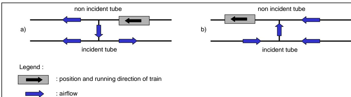
Figure 7: Schematic view of the airflows induced by a running train with open cross-passages
