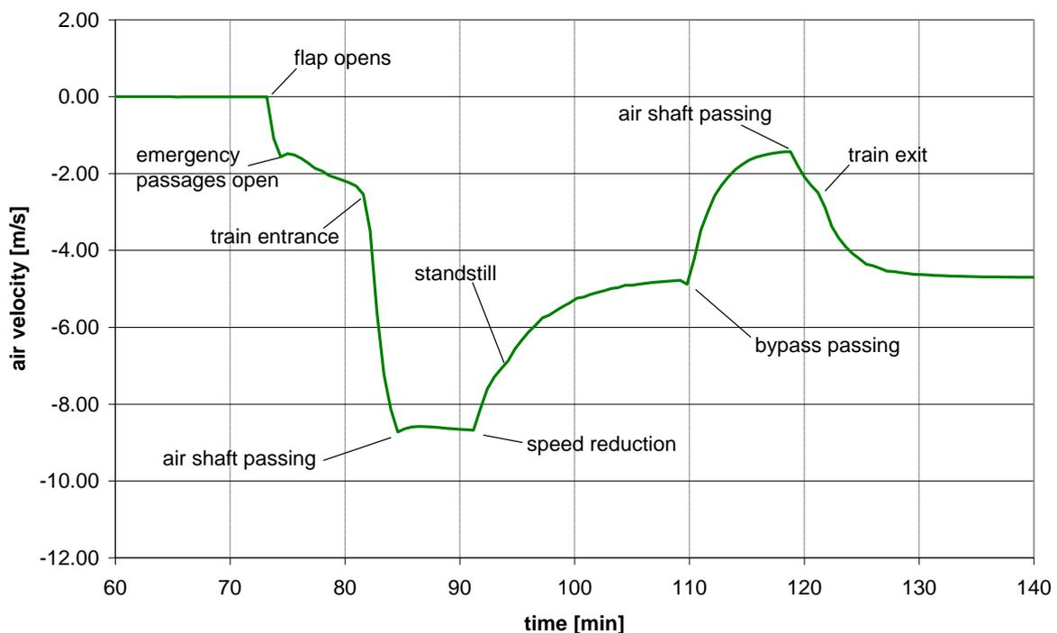
Figure 8: Simulation of the train induced airflows through an open bypass channel
