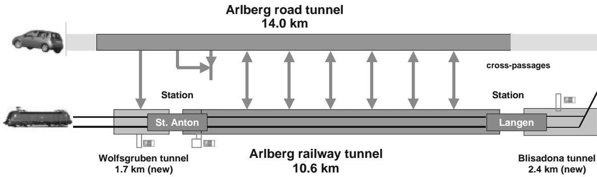
**Fig. 2: Arlberg tunnel – Cross-passages between road and railway tunnel**
