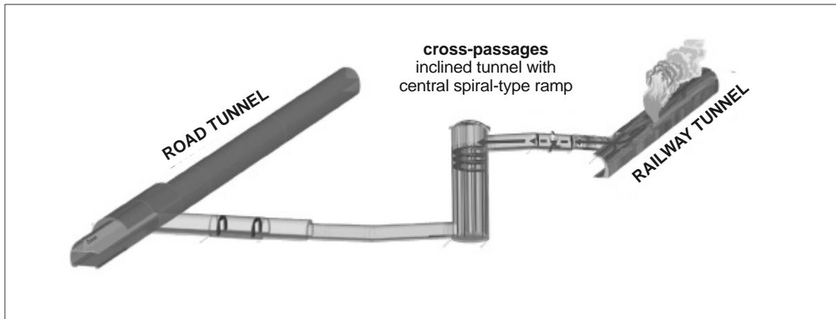
**Fig. 4: Cross-passage with spiral-type ramp**
