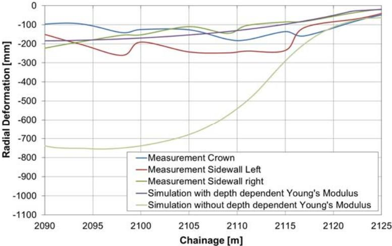
**Figure 4. Measurement results and results from simulation**
