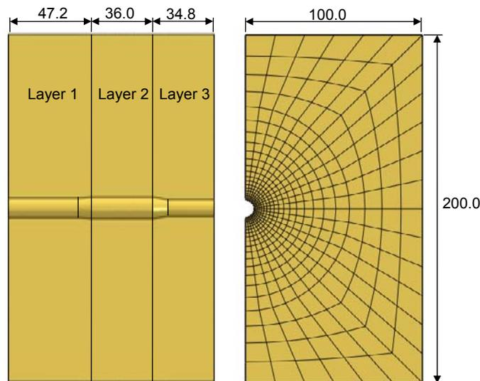
Figure 2. a) Front view of the model including dimensions; b) side view of the model including dimensions and mesh
