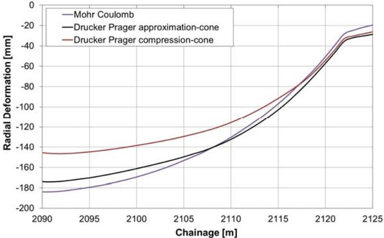
**Figure 5. Results for simulations with a Mohr Coulomb and a Drucker Prager failure criterion**
