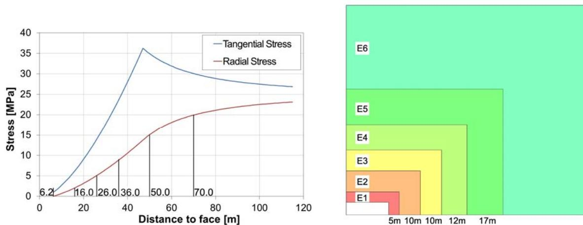
**Figure 3. a) Determination of the distance to the tunnel perimeter; b) Distribution of the different Young's moduli in the numerical model**
