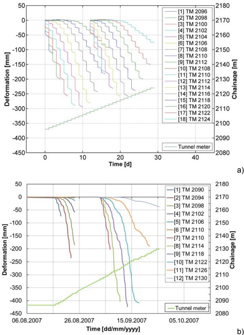
Figure 6. a) Axial extrusion in front of the face (simulation results); b) measurement results from RH-Extensometers
