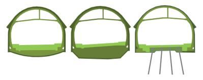
Figure 3. Cross sections in sections with swelling heave: left: Zone DZ I; center: DZ III with invert slab, right: DZ II with tiebacks
