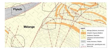
Figure 2. The complex geological structure at Gotschna tunnel showing different geotechnical situations for different tunnel sections (Krähenbühl, 2014)
