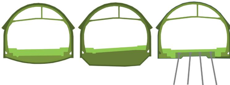
Figure 3. Cross sections in sections with swelling heave: left: Zone DZ I; center: DZ III with invert slab, right: DZ II with tiebacks
