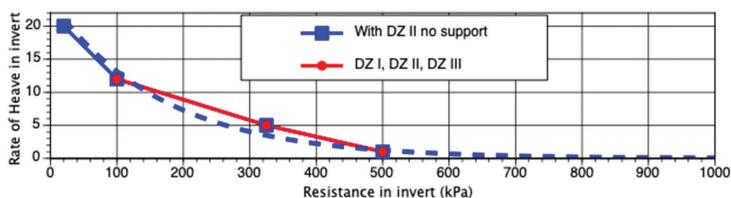
Figure 4. Rate of deformation vs. support pressure of invert for Gotschna tunnel with exponential correlation (—) through four points and linear correlation (---) through 3 points.
