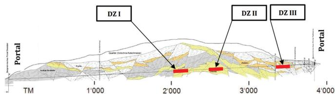
Figure 1. Geologic conditions along Gotschnatunnel (Krähenbühl, 2014) with swelling zone 1 (DZ I), zone 2 (DZ II) with anchors in the invert and zone 3 (DZ3) with invert.
