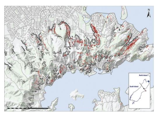
Figure 2 The Port Hills road network and the extent of boulder release (dots and thicker dark lines) during the 2010/2011 earthquake sequence. Sources: Land Information New Zealand 2015, CCC n.d.
