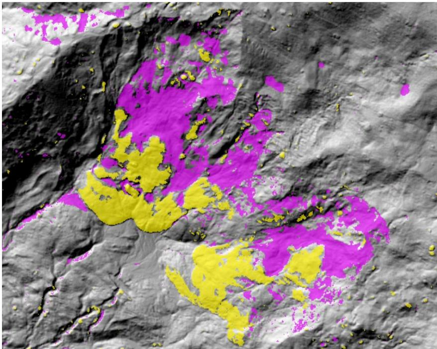
Further information on terrain (in-)stability can be derived from satellite-borne interferometric synthetic aperture radar (InSAR) data (e.g. Rott & Nagler 2006). Multi-temporal radar images cover large areas (up to hundreds of km<sup>2</sup>) and can provide information on locations and amounts of ground deformations (landslide and earthquake displacement maps; see Figure 2).
