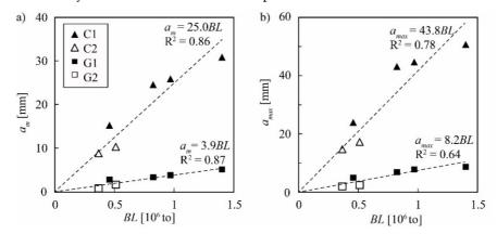
**Figure 10.** (a) Mean and (b) maximum cumulative abrasion depths as a function of cumulative bedload mass at Pfaffensprung SBT for high-strength concrete test fields C1 and C2 and granite test fields G1 and G2 for the years 2012 to 2015.
