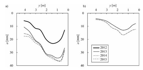
**Figure 9.** Super-elevated longitudinally averaged cross-sectional abrasion profiles of high-strength concrete test fields (a) C1 at test location 1 and (b) C2 at test location 2 installed at Pfaffensprung SBT for the years 2012 to 2015; view in flow direction.
