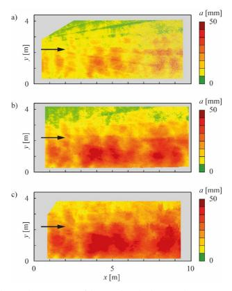
**Figure 5.** High-resolution abrasion maps of the 10 m long high-strength concrete test field C1 installed at test location 1 in Pfaffensprung SBT after (a) one, (b) two and (c) four operational years (the grey colored areas could not be scanned due to ground water drainage installation).
