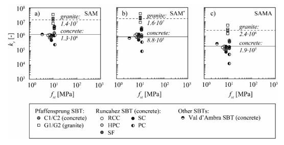
**Figure 14.** Abrasion coefficient  $k_v$  as a function of splitting tensile strength of various SBT invert materials for (a) SAM, (b) SAM\* and (c) SAMA.
