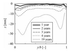
**Figure 12.** Super-elevated, longitudinally averaged cross-sectional abrasion profiles of the silica fume concrete test field (SC) in Runcahez SBT.
