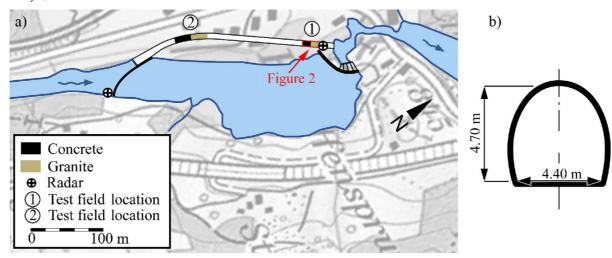
**Figure 1.** (a) Overview and (b) cross section of the Pfaffensprung SBT (position 46°42′49.8″ N 8°36′36.7″ E) with test field locations 1 and 2 and radar instrumentation for discharge monitoring, position of Figure 2 highlighted red.
