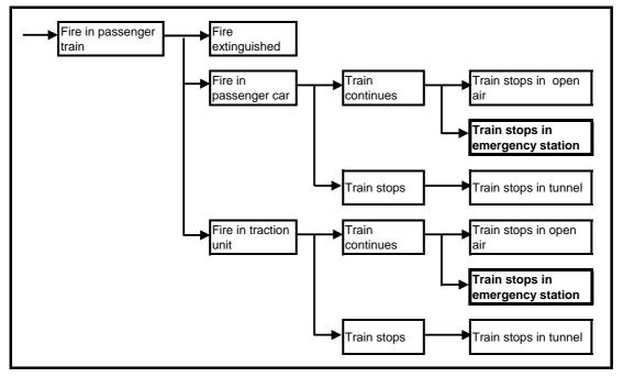
Figure 3: Simplified event tree for fire in passenger train
