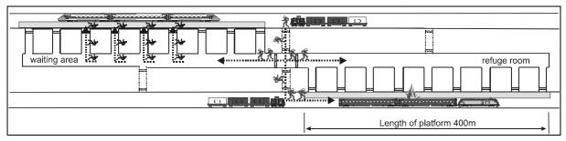
Figure 5: Evacuation train and rescue train in emergency station
