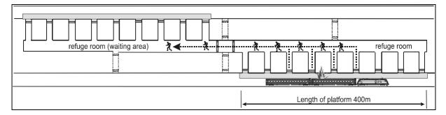
Figure 4: Layout of emergency station
