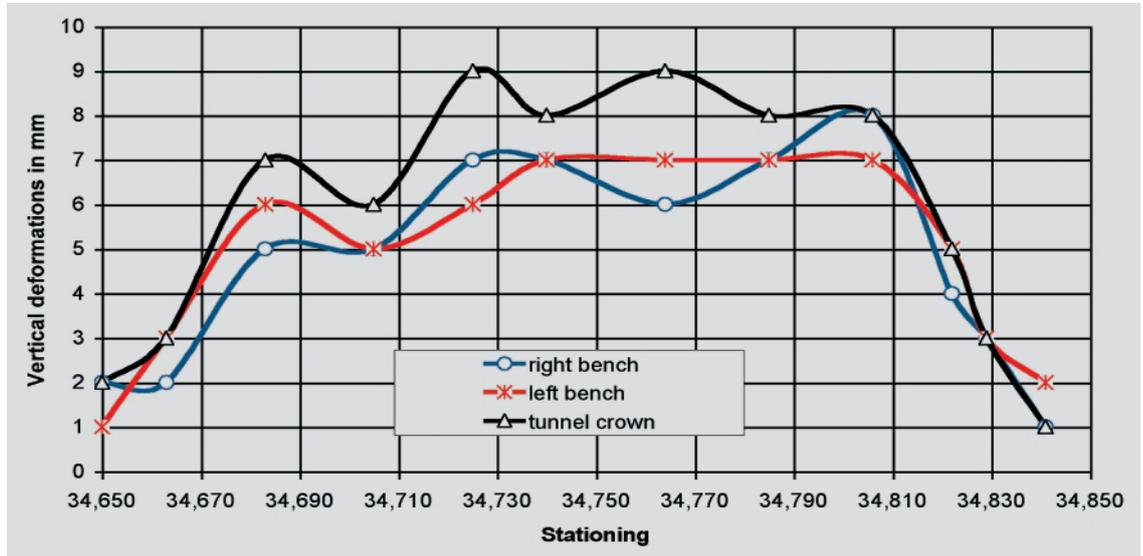
**Fig. 8** Vertical deformations related to the open cut ("+" = heave).
