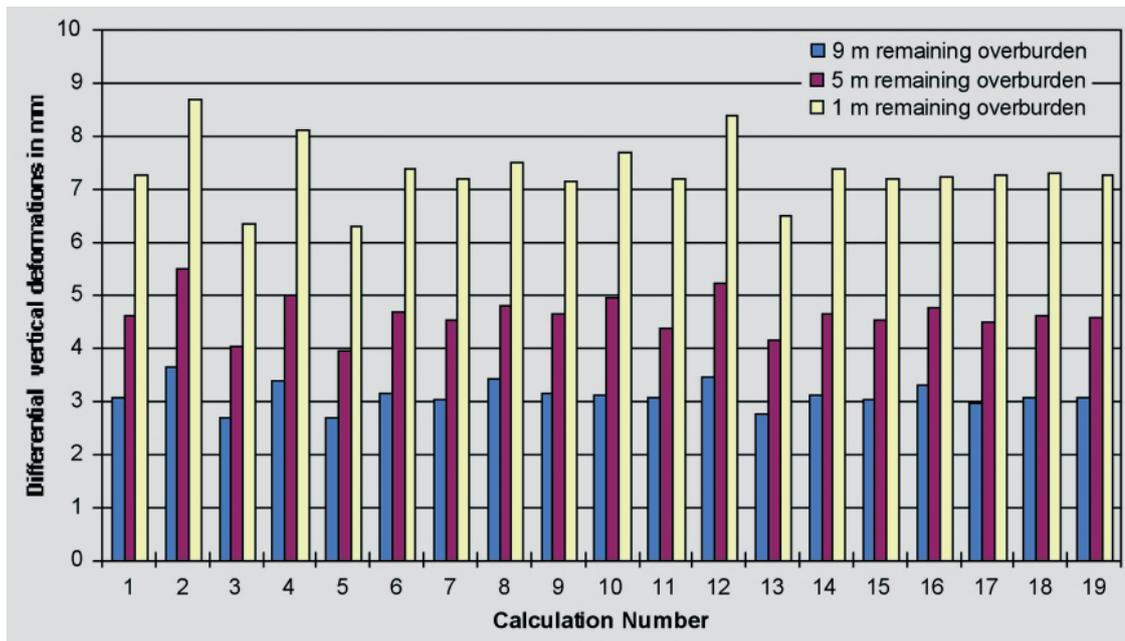
**Fig. 6** Differential vertical deformations between tunnel crown and invert.
