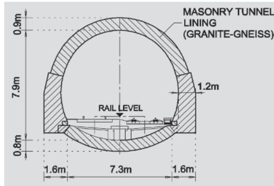
Fig. 2 Tunnel lining.
