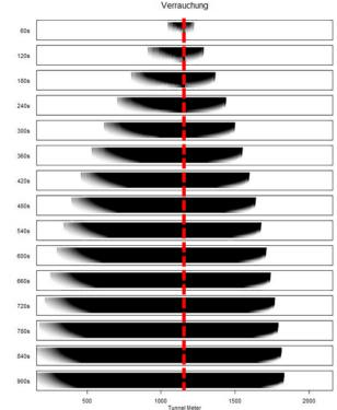
Longitudinal smoke propagation for a corresponding airflow velocity of -0,5m/sec.
