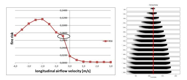
Fig. 6: Detailed results: fire risk (traffic volume 400veh/h) in dependence of longitudinal airflow velocity and smoke propagation for a longitudinal airflow of -0,5 m/s
