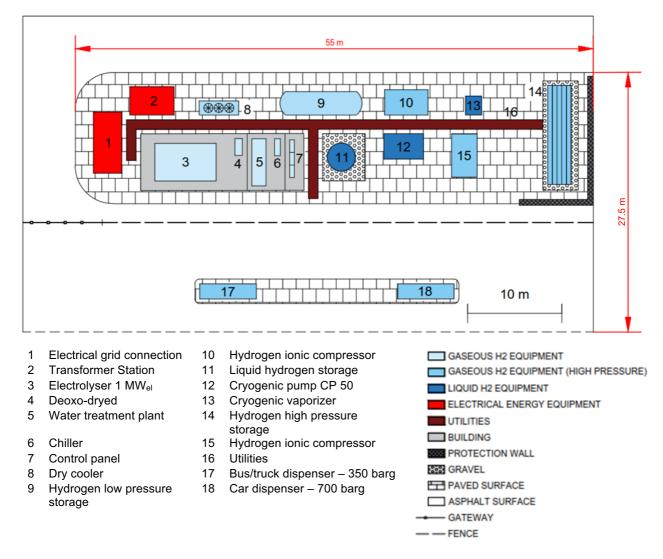
Figure 2 Layout of a fuelling station with electrolyser
