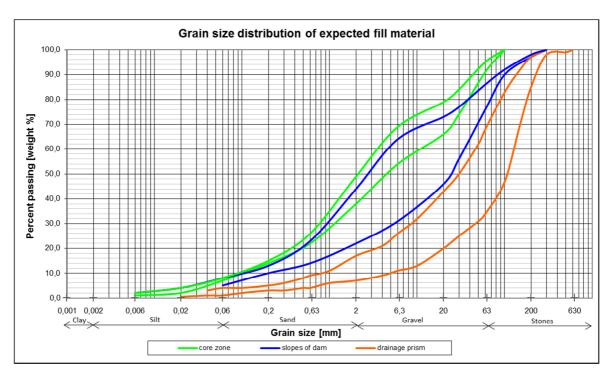
Figure 7: Estimated upper (favourable) and lower (non-favourable) boundary of grain size distribution of expected dam fill materials; green: core zone of dam, blue: slope of dams, orange: drainage prism.
