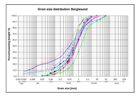
Figure 2: Grain size distributions of the "Berglesand", excavated in trial pits at the planned upper reservoir site.
