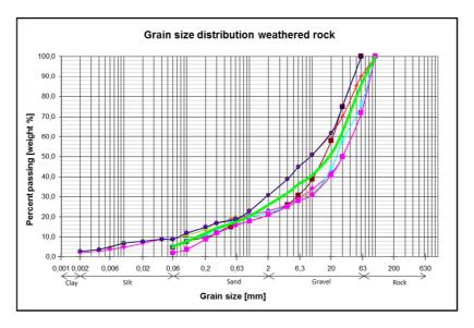
Figure 3: Grain size distributions of weathered rocks, excavated in trial pits at the planned upper reservoir.
