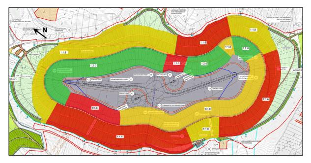
Figure 5: Layout of the upper basin ring dam with different slope inclinations coloured red (1:1.6), green (1:1.8) and yellow (1:2.0).
