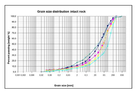
Figure 4: Grain size distributions of excavation material from intact rocks (paragneisses, granites), encountered in the investigation adit for the Atdorf cavern.
