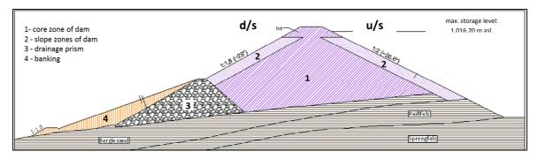
*Figure 6: Cross section of the planned dam; d/s-downstream side; u/s – upstream side.*
