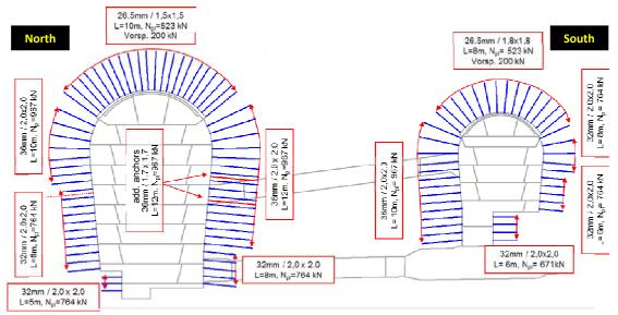
Figure 10. Final anchor support system
