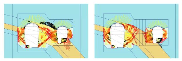
Figure 3. Development of plastic zones - cavern axis distance (62 m versus 82 m)
