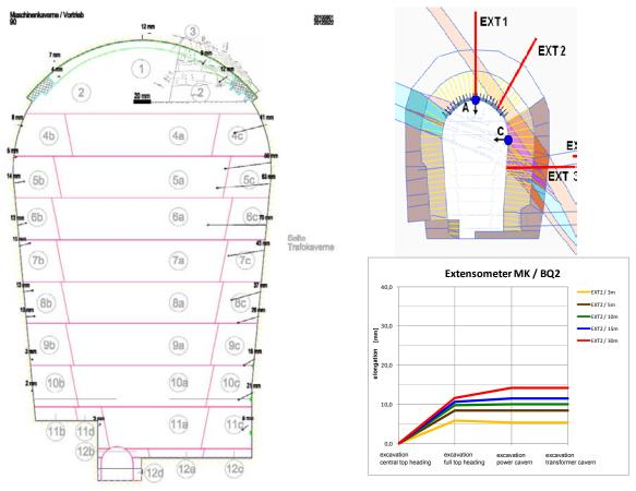
Figure 9. Side wall deformation data of the critical section
