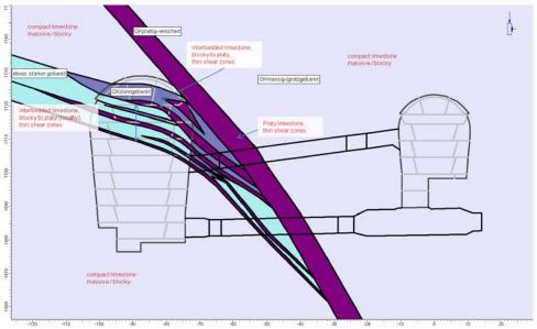
Figure 8. Refined model of the weak zone as updated during excavation
