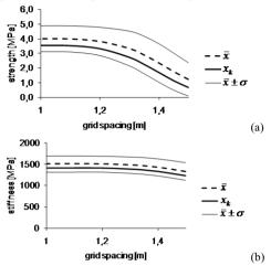
Figure 10. Key values of (a) strength and (b) stiffness plotted against the grid spacing.
