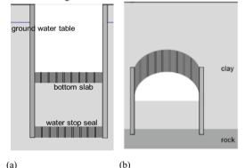
Figure 3. Different applications of jet grouting measures: (a) deep excavation (b) temporary support in tunnelling using NATM.
