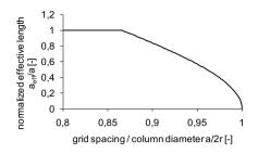
Figure 5. Analytical result of normalized effective contact length as a function of the grid spacing normalized with the column diameter.
