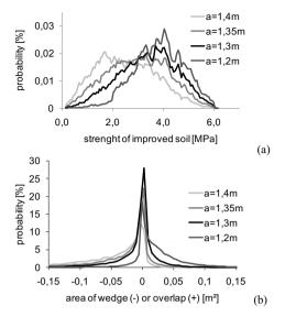
Figure 9. Results from variation of the grid spacing between 1,2 m and 1,4 m (a) strength; (b) wedge size.
