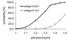
Figure 11. Probability of existence of a wedge  $(>0,0m^2)$  and of wedges exceeding the size of  $0,1m^2$  plotted against the grid spacing.
