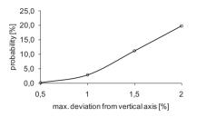
Figure 13. Probability of wedge sizes exceeding 0,1m<sup>2</sup> plotted against maximum deviation from verticality.
