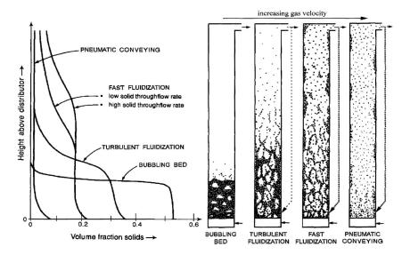
Fig. 3: Typical distribution of solids in various fluidization regimes (merged figure from [16–18])
