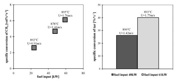
Fig. 6: Specific hydrocarbon conversions in the DCFB pilot plant: CH<sub>4</sub> conversion (left) and conversion of total amount of tar (right), model tar substance: 1-methylnaphthalene
