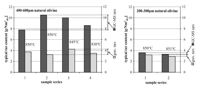
Fig. 5: Tar content in the product gas of the 100 kW DFB gasifier with two different batches of bed material
