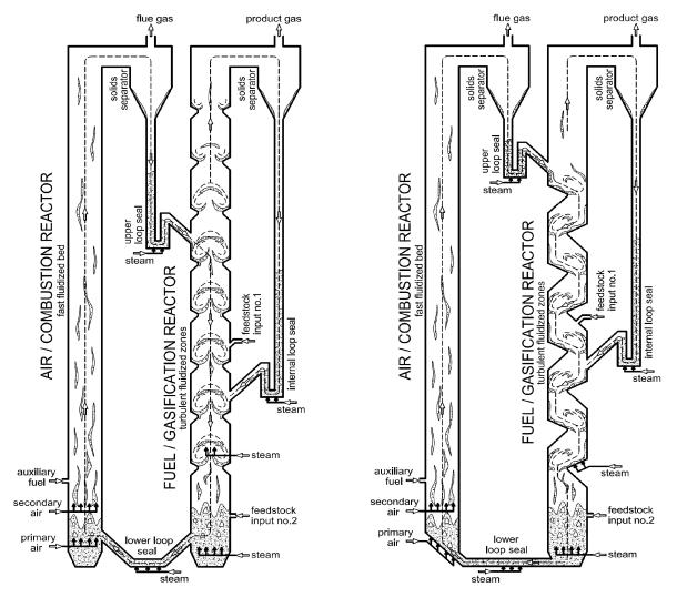
Fig. 12: Novel dual circulating fluidized bed concept with gas-solids counter-current flow: Two possible designs
