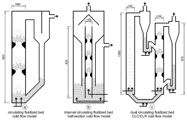
Fig. 4: Cold flow models used for the characterization of obstacle effects
