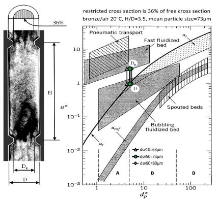
Fig. 9: Flow conditions in fuel reactor with constrictions [16, 18]
