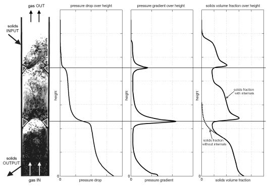
Fig. 8: Typical qualitative pressure drop, pressure gradient, and solids fraction in the fuel reactor with zones of improved gas-solid interaction
