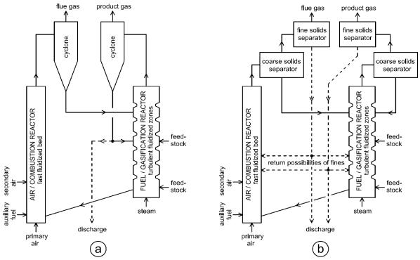
Fig. 13: Gas-solid separator arrangement and possible return paths of solids
