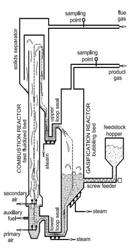
Fig. 1: Classical DFB configuration (100 kW gasifier pilot plant as example)
