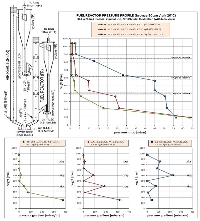
Fig. 11: Pressure drop and pressure gradient of a fuel reactor with ring type internals. FR = fuel reactor, AR = air reactor, ULS = upper loop seal, LLS = lower loop seal, ILS = internal loop seal
