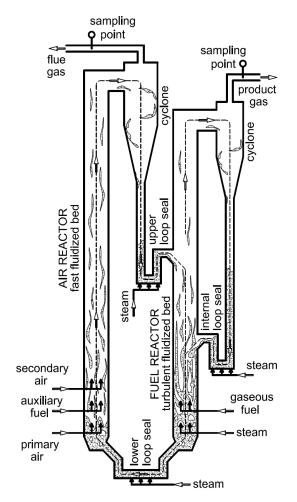
Fig. 2: Dual circulating fluidized bed (DCFB) system (120 kW pilot unit as example)
