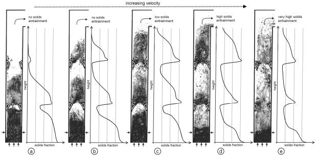
Fig. 7: Flow conditions and solids fraction in the fuel reactor with zones of improved gas-solid interaction
