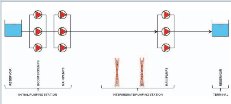
FIGURE 3: Closed pipeline system
