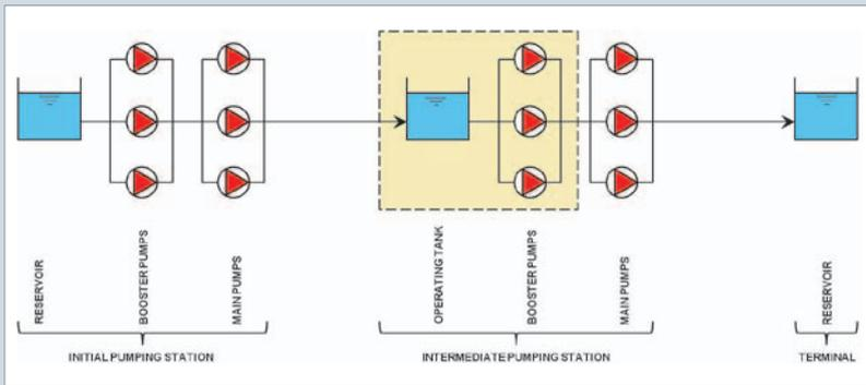
FIGURE 2: Open pipeline system
