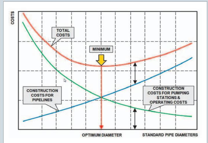
FIGURE 9: Pipeline diameter optimisation
