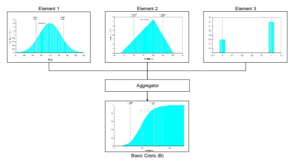
Figure 3: Schematic determination of basic costs using a probabilistic approach
