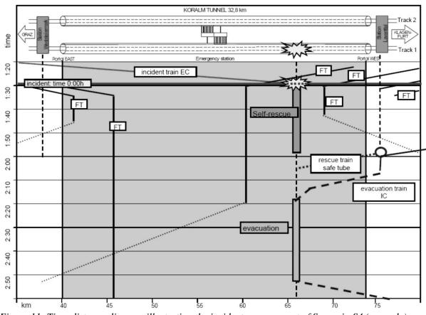
Figure 11: Time-distance diagram illustrating the incident management of Scenario S4 (example)
