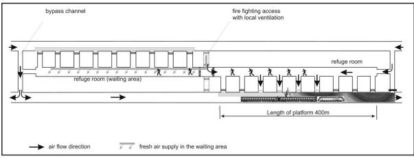
*Figure 6: Air flow direction in case of self-rescue (open doors at the escape passages) in the emergency station*
