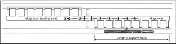
Figure 3: Layout of emergency station
