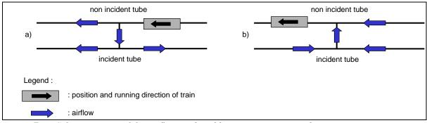
Figure 7: Schematic view of the airflows induced by a running train with open cross-passages
