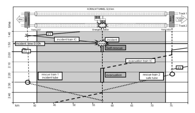
Figure 10: Time-distance diagram illustrating the incident management of Scenario S1 (example)
