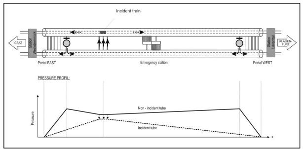
*Figure 5:* Airflows and pressure profile in an emergency situation with a train coming to a halt outside the emergency station
