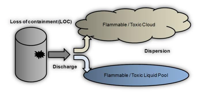
Figure 3 Discharge and dispersion following a loss of containment (LOC)
