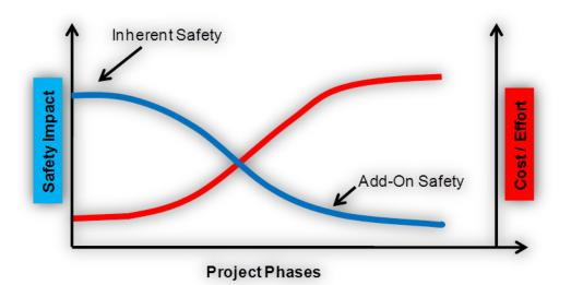
Figure 1 Safety impact and cost of risk reducing measures during a project
