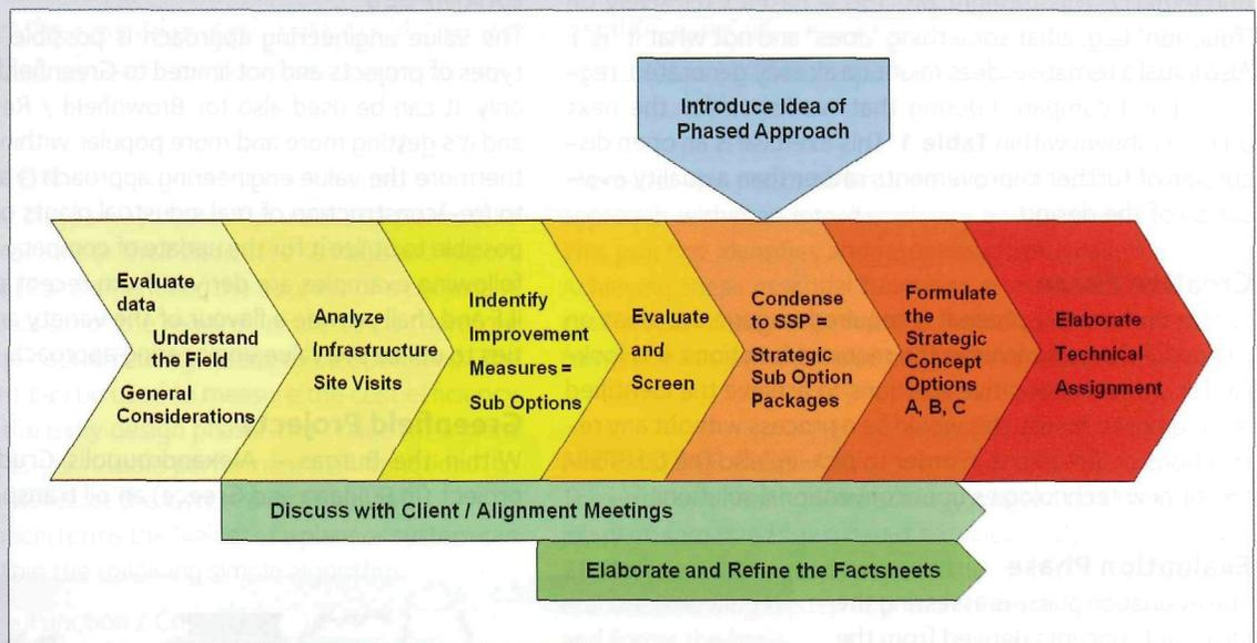
FIGURE 3: Value engineering workflow within re-engineering project
