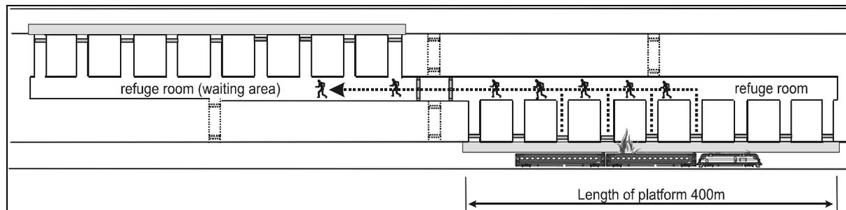
**Figure 4: Layout of emergency station**
