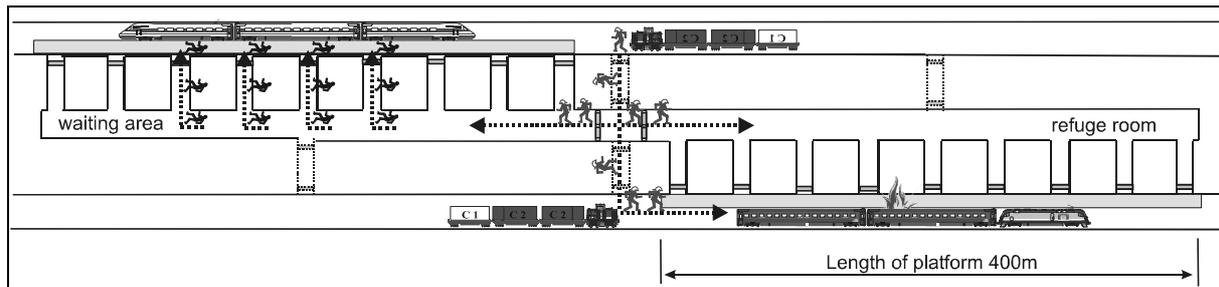
**Figure 5: Evacuation train and rescue train in emergency station**
