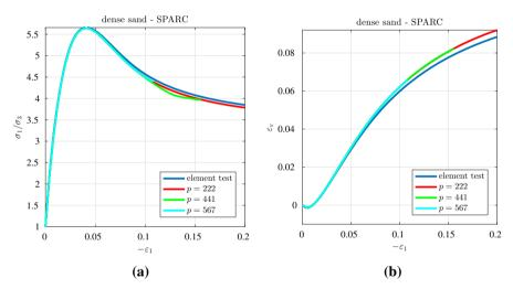
Fig. 21 Dense triaxial test—comparison of element test and 3D SPARC simulations for simulation setup I: stress-strain-curve (a) and volumetric-axial-strain-curve (b)
