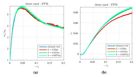
Fig. 11 Dense triaxial test—comparison of element test and 3D FPM simulations for simulation setup I: stress-strain-curve (a) and volumetric-axial-strain-curve (b)
