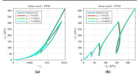
Fig. 7 Dense oedometric test—comparison of element test and 3D FPM simulations for simulation setup II: stress-strain-curve (a) and stress path (b)
