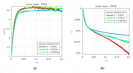
Fig. 13 Loose triaxial test—comparison of element test and 3D FPM simulations for simulation setup I: stress-strain-curve (a) and volumetric-axial-strain-curve (b)
