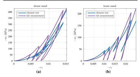
Fig. 3 Oedometric test-comparison of lab measurement and element test: stress-strain-curves for dense (a) and loose sand (b)
