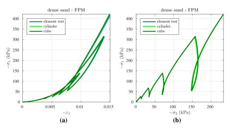
**Fig. 8** Dense oedometric test—comparison of element test and 3D FPM simulations for different geometrical bases ( $v_p = \pm 0.001 \text{ m/s}$ ,  $\Delta t = 0.0009 \text{ s}$ , and h = 0.01 m): stress-strain-curve (**a**) and stress path (**b**)
