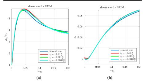
Fig. 12 Dense triaxial test—comparison of element test and 3D FPM simulations for simulation setup II: stress-strain-curve (a) and volumetric-axial-strain-curve (b)
