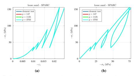
Fig. 17 Loose oedometric test—comparison of element test and 3D SPARC simulations for simulation setup I: stress-strain-curve (a) and stress path (b)
