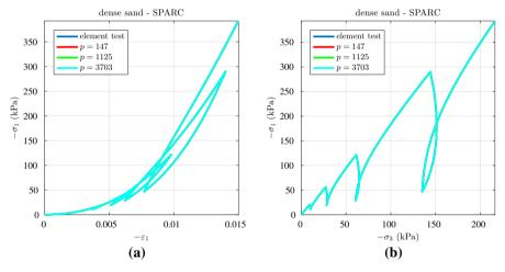
Fig. 15 *Dense oedometric test*—comparison of element test and 3D SPARC simulations for simulation setup I: stress-strain-curve (**a**) and stress path (**b**)
