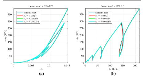
Fig. 16 Dense oedometric test—comparison of element test and 3D SPARC simulations for simulation setup II: stress-strain-curve (a) and stress path (b)
