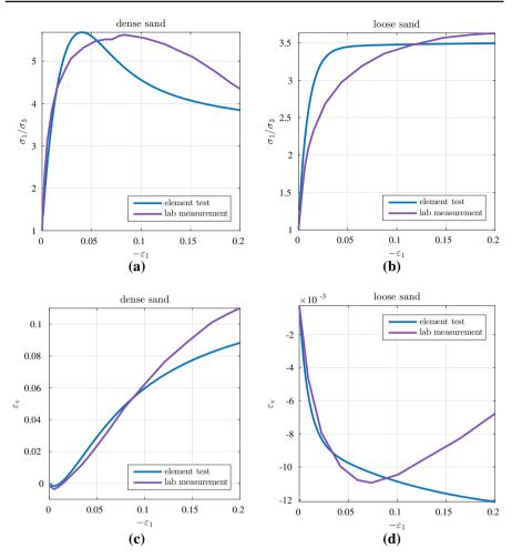
**Fig. 4** *Triaxial test*—comparison of lab measurement and element test for dense (**a**, **c**) and loose sand (**b**, **d**): stress-strain-curve (first row) and volumetric-axial-strain-curve (second row)
