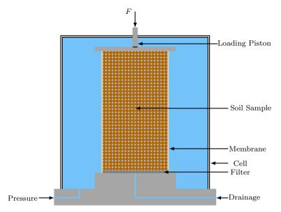
Fig. 2 Schematic illustration of the triaxial test
