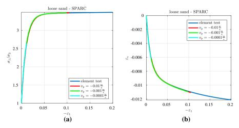
Fig. 24 Loose triaxial test—comparison of element test and 3D SPARC simulations for simulation setup II: stress-strain-curve (a) and volumetric-axial-strain-curve (b)
