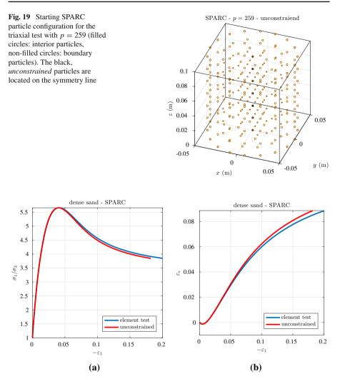
Fig. 20 Comparison of element test and 3D SPARC simulation for the *unconstrained* triaxial test with dense sand (p = 259,  $v_p = -0.01$  m/s, and  $\Delta t = 0.01$  s): stress-strain-curve (**a**) and volumetric-axial-strain-curve (**b**)
