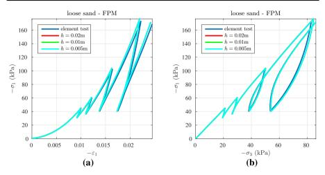
Fig. 9 Loose oedometric test—comparison of element test and 3D FPM simulations for simulation setup I: stress-strain-curve (a) and stress path (b)
