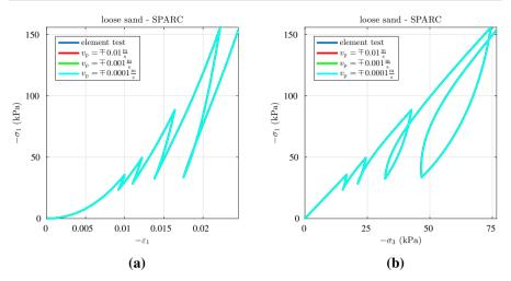
Fig. 18 Loose oedometric test—comparison of element test and 3D SPARC simulations for simulation setup II: stress-strain-curve (a) and stress path (b)
