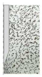
Figure 4.8: Displacement vectors of particles obtained by discrete element method (adapted from Zöhrer [63])
