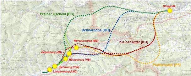
Figure 3 – Semmering base tunnel: route alternatives and different locations of portal station in Styria
