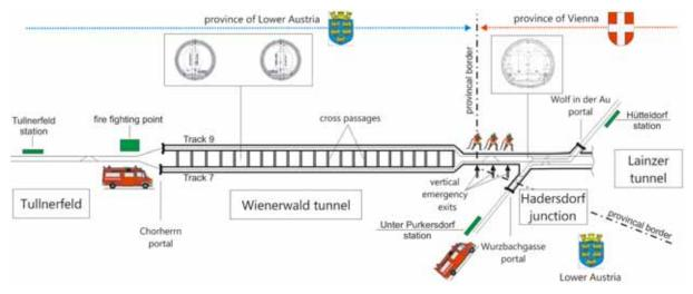
Figure 2: Change of tunnel system within the Wienerwald tunnel
