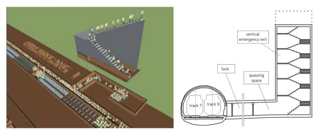
Figure 4: Evacuation simulation of vertical emergency exits
