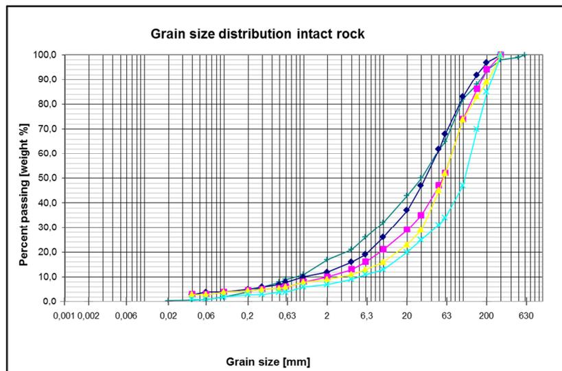
Figure 4: Grain size distributions of excavation material from intact rocks (paragneisses, granites), encountered in the investigation adit for the Atdorf cavern.
