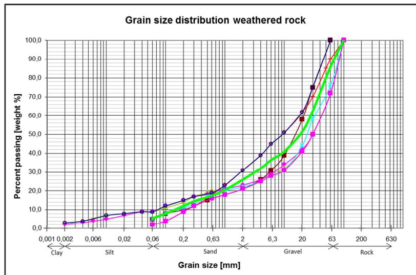
Figure 3: Grain size distributions of weathered rocks, excavated in trial pits at the planned upper reservoir.
