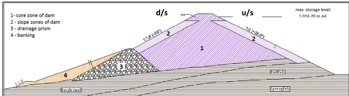
Figure 6: Cross section of the planned dam; d/s – downstream side; u/s – upstream side.
