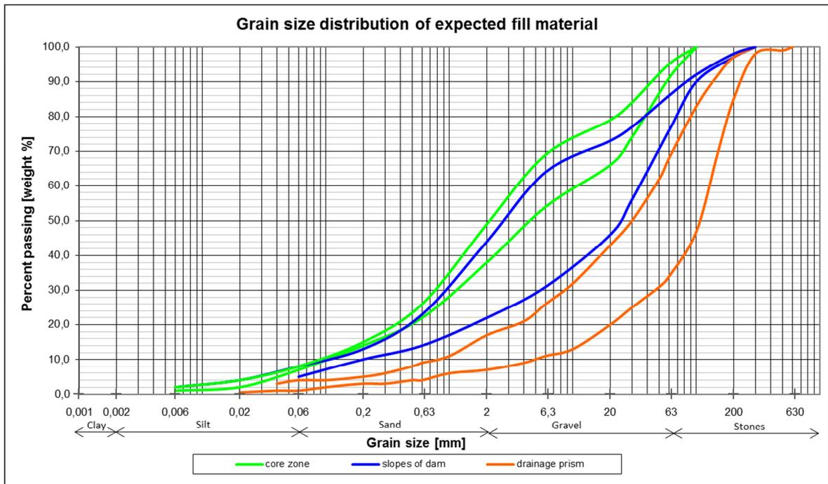
Figure 7: Estimated upper (favourable) and lower (non-favourable) boundary of grain size distribution of expected dam fill materials; green: core zone of dam, blue: slope of dams, orange: drainage prism.
