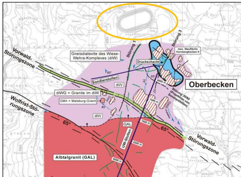
Figure 1: Structural setting of the existing reservoir (Hornbergbecken, highlighted in yellow), the investigation tunnel (Sondierstollen), and the planned facilities of the upper reservoir (Oberbecken) and tailrace tunnel (UW-Stollen). Extract from Franzke (2012). Violet: Wiese-Wehra paragneiss complex (diW). Red: Granites (Albtal granite GAL). Black and green lines: major fault zones. Extract from Schluchseewerk (2014; and Franzke 2012 resp.).
