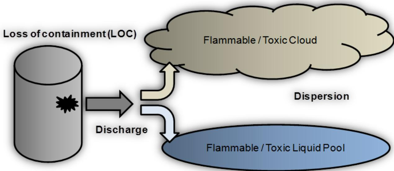
Figure 3 Discharge and dispersion following a loss of containment (LOC)
