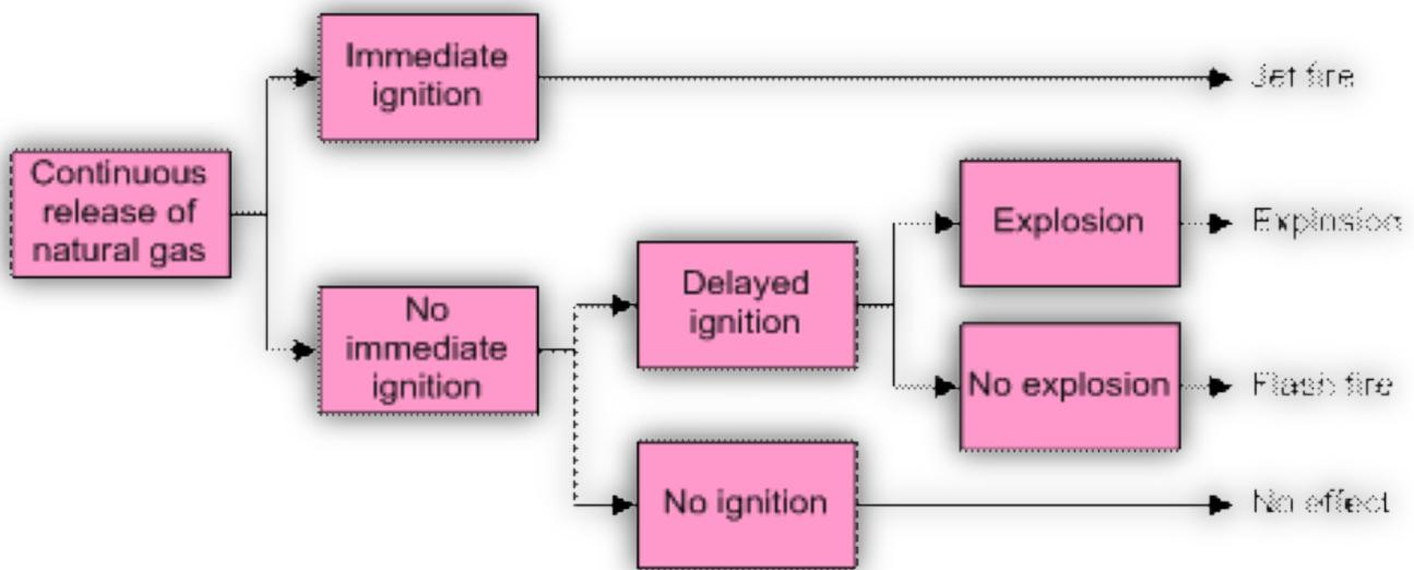
Figure 2 Event tree for a continuous release of pressurized natural gas
