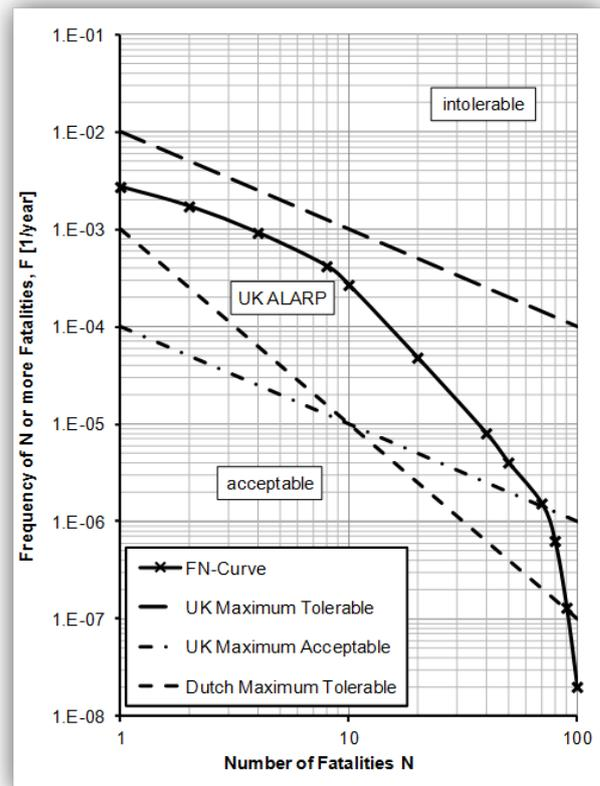
Figure 7 Typical FN-curve
