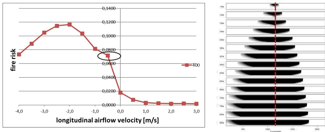
Fig. 6: Detailed results: fire risk (traffic volume 400veh/h) in dependence of longitudinal airflow velocity and smoke propagation for a longitudinal airflow of -0,5 m/s
