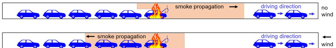
Fig. 3: Change of smoke propagation direction in case of extreme wind on the tunnel portal
