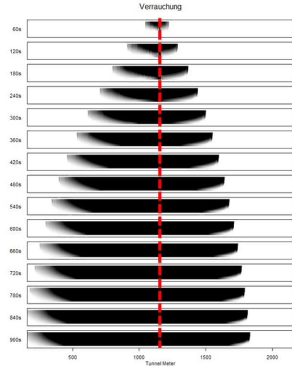
Longitudinal smoke propagation for a corresponding airflow velocity of -0,5m/sec.
