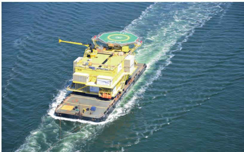
Figure 3.1.6.1: Transporting a transformer substation for a wind farm in the North Sea. | Source: Dr. Born - Dr. Ermel GmbH.
