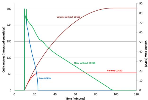
**Figure 1.** An example of the spill volumes on a downhill section of pipeline with a 2 in. leak hole.
