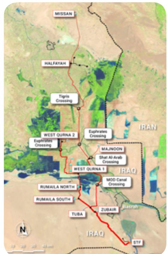
> CSSP Pipeline Routing Overlay onto the Iraq Satellite Image
