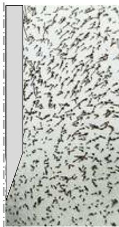
Figure 4.8: Displacement vectors of particles obtained by discrete element method (adapted from Zöhrer [63])
