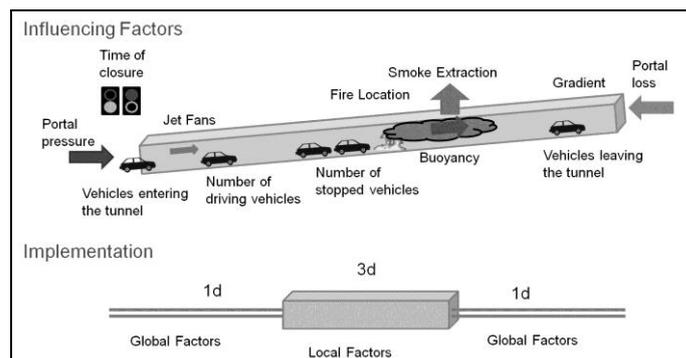
Figure 8. Influencing factors taken into account in the new 1D / 3D smoke propagation model of RVS 09.03.11 [9]
