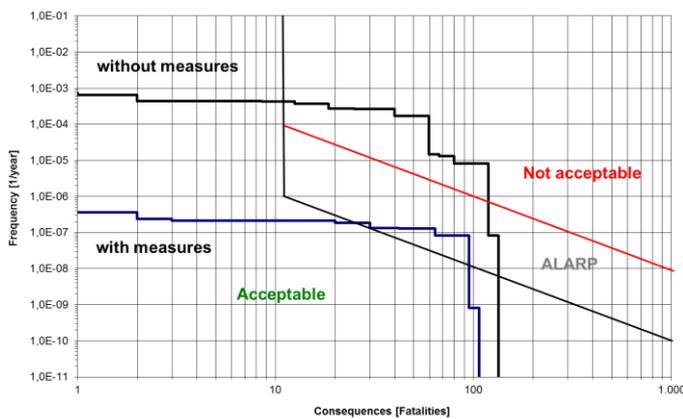
Figure 6. FN diagram including absolute criteria of acceptability
