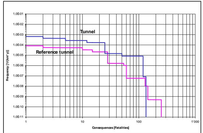
Figure 7. comparison of FN curves of “real” tunnel and “reference tunnel”
