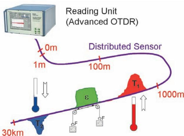
Fig. 3: Temperature and strain profiles along optical fiber
