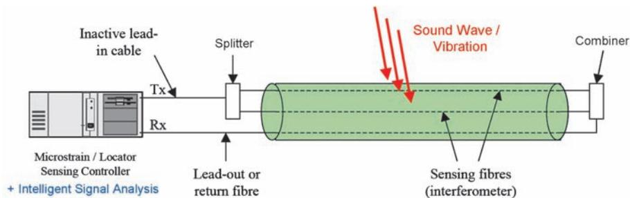
**Fig. 4:** System block diagram presenting fiber optic interferometer
