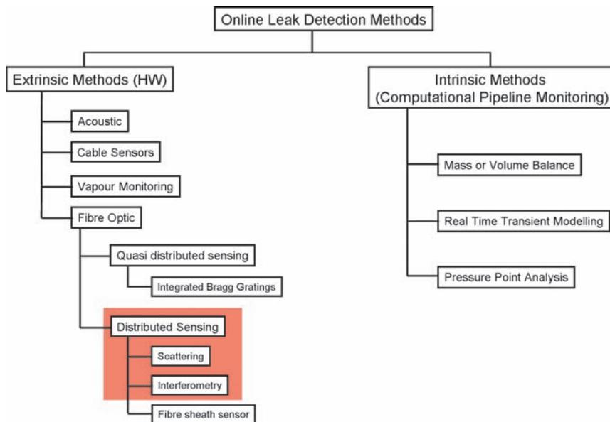
**Fig. 1:** Online Leak Detection Methods
