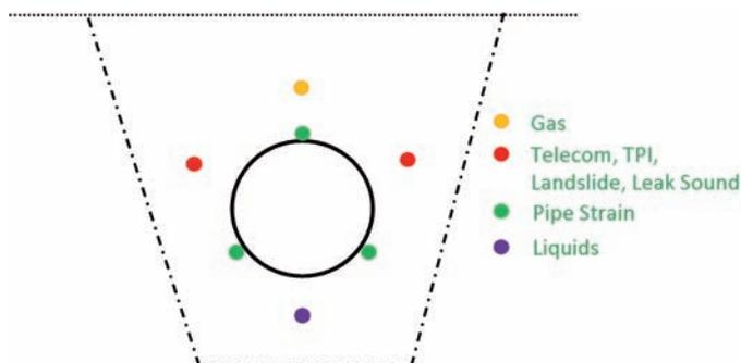
**Fig. 5:** Application Specific Locations for Fiber Optic Cable
