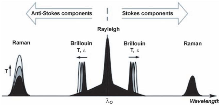
Fig. 2: Scattering effects within fiber optic cables caused by temperature [T] or strain [ε]
