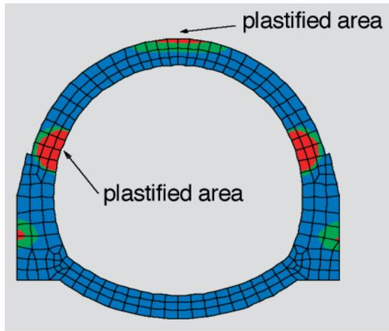
**Fig. 3** Plastified areas with a remaining overburden of 1 m.
