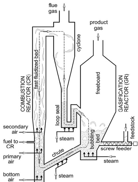
Fig.1: Classical dual fluidized bed gasifier design
