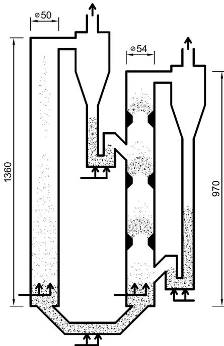
**Fig.5: DCFB CLC cold flow model used for investigations**
