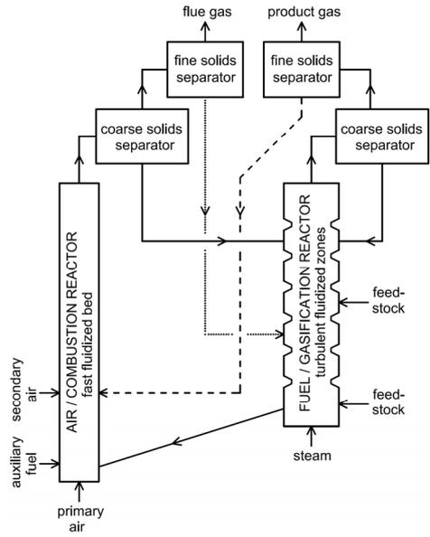
**Fig.10: Multistage gas–solid separator arrangement with return paths of coarse and fine solids**
