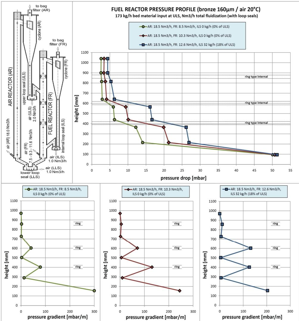
**Fig.8:** Pressure drop and gradient in the fuel (gasification) reactor of the “G-volution” system
