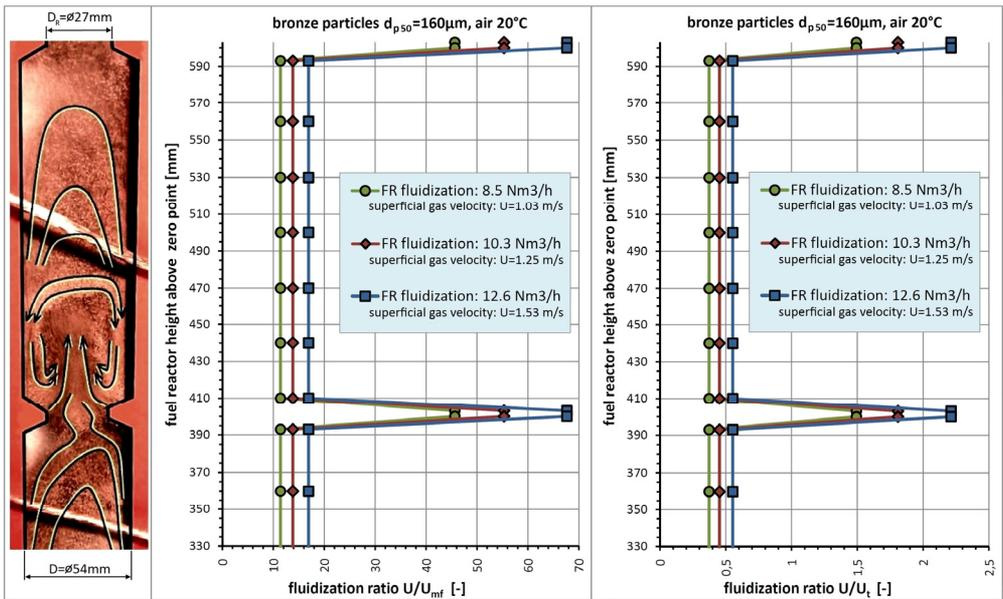
Fig.6: flow pattern and fluidization ratios in the countercurrent gasification reactor, restricted cross section = 25% of free cross section
