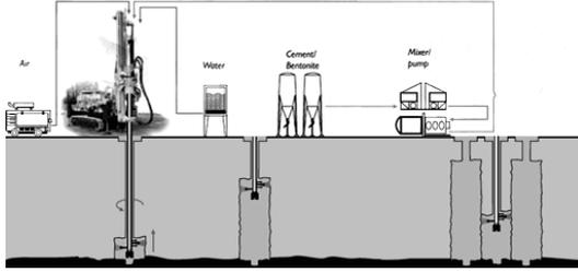
Figure 1. Principle of jet-grouting [11]
