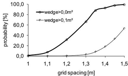
Figure 11. Probability of existence of a wedge (>0,0m²) and of wedges exceeding the size of 0,1m² plotted against the grid spacing.
