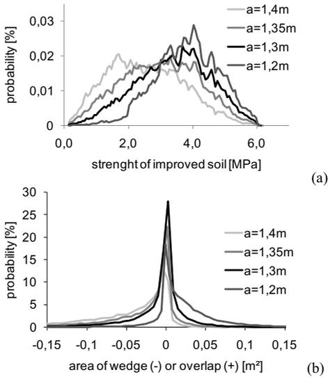
Figure 9. Results from variation of the grid spacing between 1,2 m and 1,4 m (a) strength; (b) wedge size.
