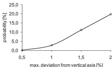
Figure 13. Probability of wedge sizes exceeding  $0,1\text{m}^2$  plotted against maximum deviation from verticality.
