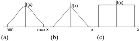
Figure 6. (a) Normal (Gauss), (b) triangular (Simpson) and (c) rectangular (uniform) distribution.
