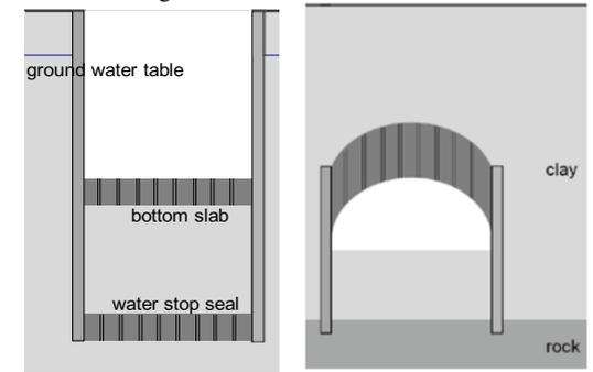
Figure 3. Different applications of jet grouting measures: (a) deep excavation (b) temporary support in tunnelling using NATM.
