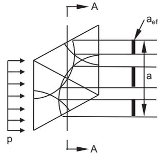
Figure 4. Effective length ( $a_{eff}$ ) for the calculation of strength in horizontal direction.
