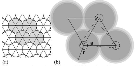
Figure 2 (a) planned grid; (b) possibilities of resulting geometries considering diameter variation and drill tolerances.
