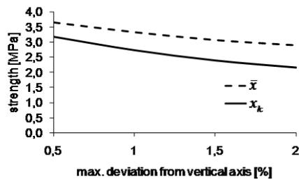
Figure 12. Strength as a function of maximum deviation from verticality of borehole.
