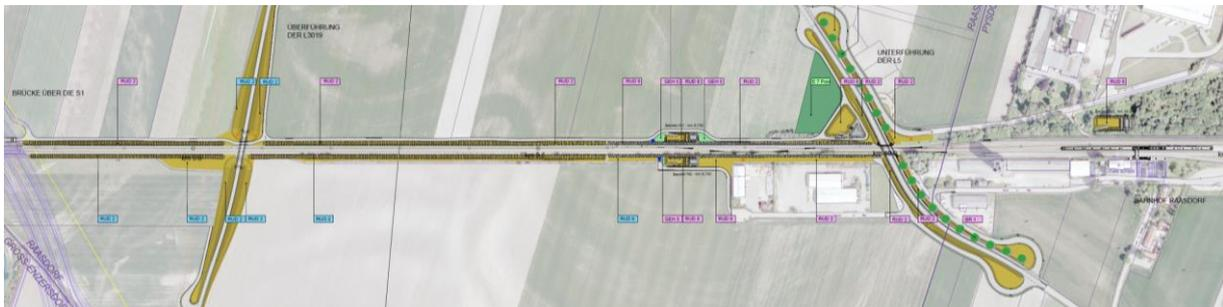
Figure 4 – Doubling of Stadlau-Marchegg railway line: secondary structures and protection and compensation measures (habitats etc.). The integrated project elaborated in this phase is the basis for the preparation of the permit application documents.
