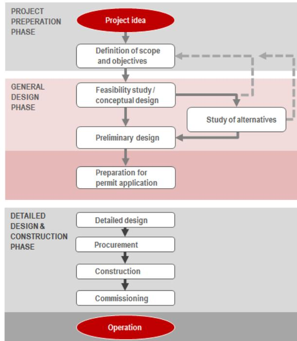
Figure 2 – Design process for a rail infrastructure project
