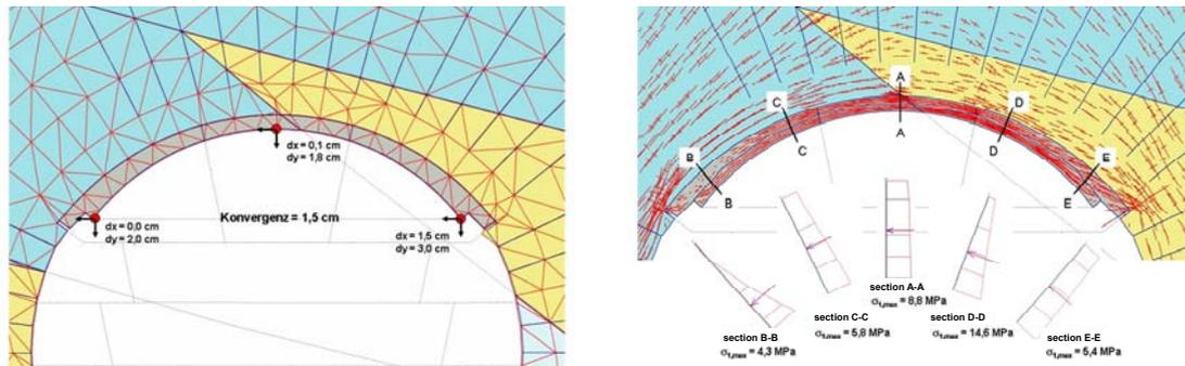
Figure 5. Concrete arch roof design – machine cavern
