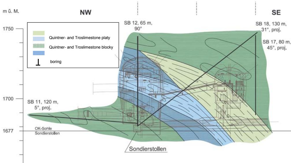
Figure 1. Typical geological cross section of main caverns (basic design with 39 m cavern spacing)
