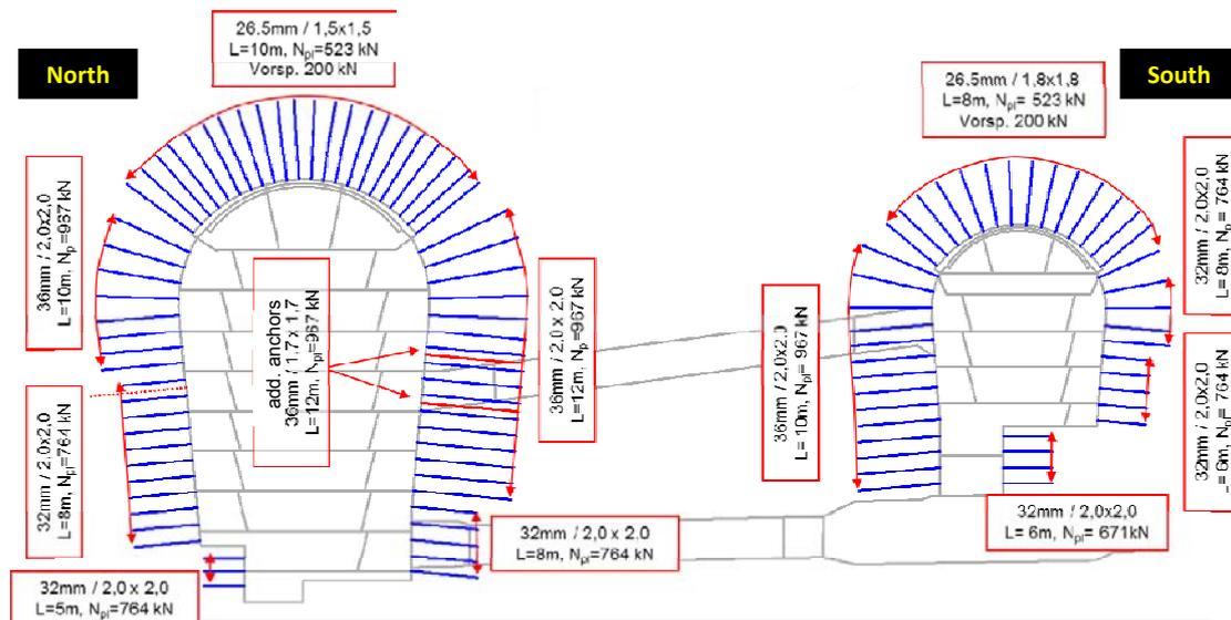
Figure 10. Final anchor support system
