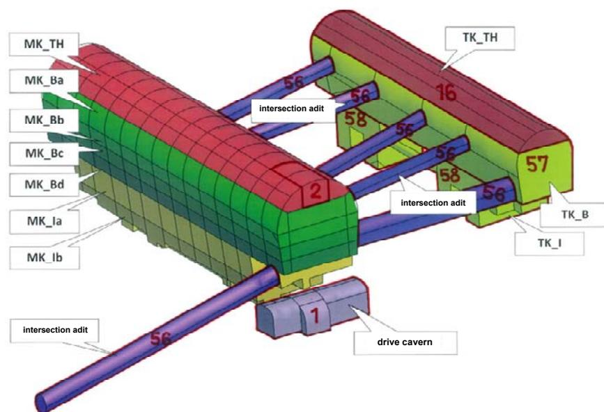
Figure 6. Full 3D FEM modelling (excavation body visualized)
