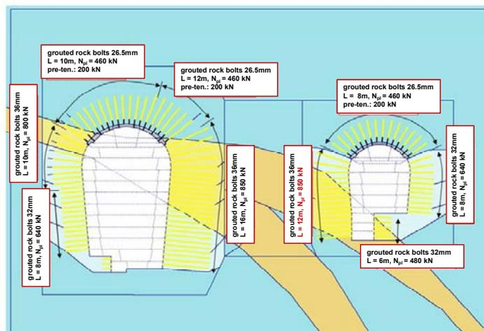
**Figure 4. Optimized support system – cavern axis distance 82 m**
