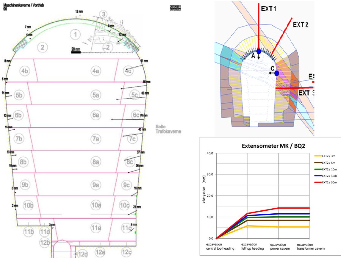
Figure 9. Side wall deformation data of the critical section
