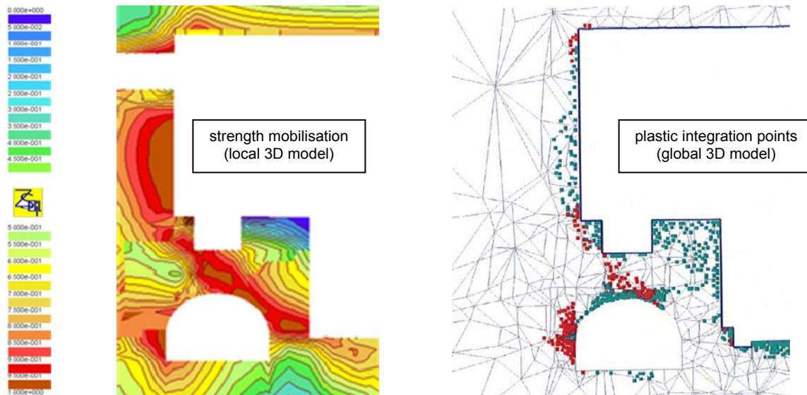
Figure 7. Comparison of different models for the interaction of the machine and the cable car cavern
