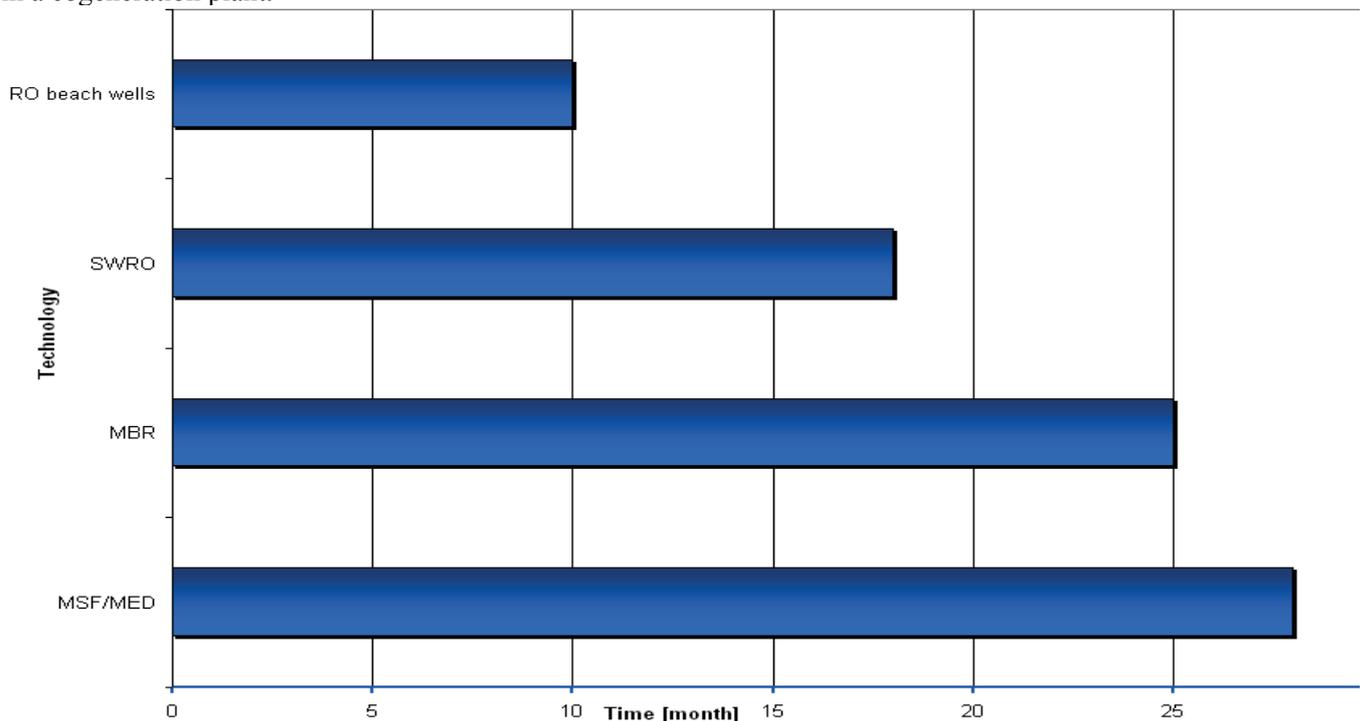
**Figure 6.18: typical construction times for different desalination technologies**
