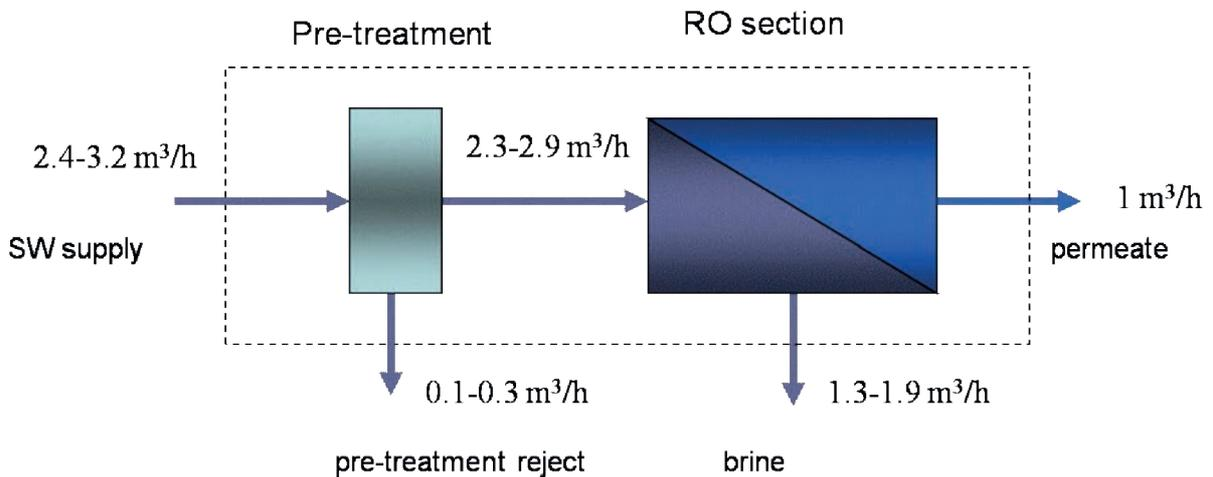
**Figure 6.2: seawater requirement SWRO process typical flow sheet**
