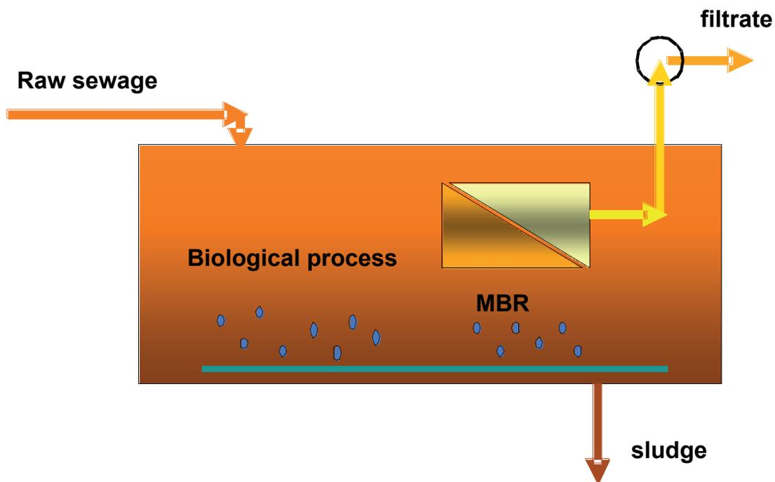
Figure 5.12 vacuum type submerged MBR
