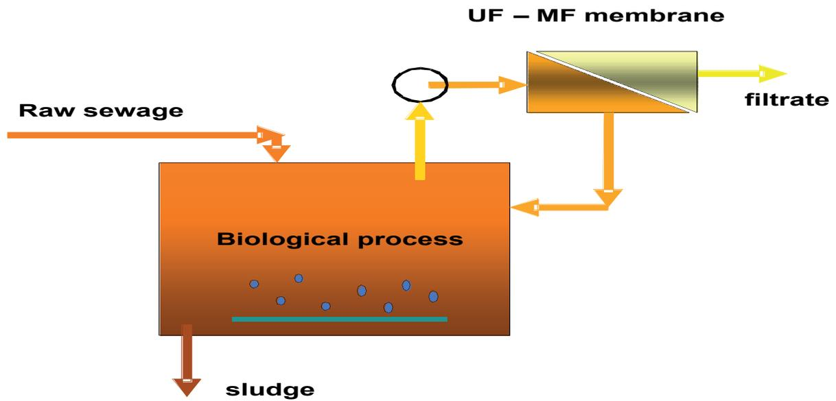
Figure 5.111 side stream waste water pressure system
