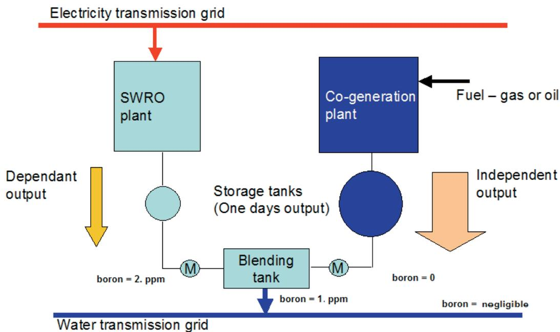
**Figure 5.7: Simple hybrid system**
