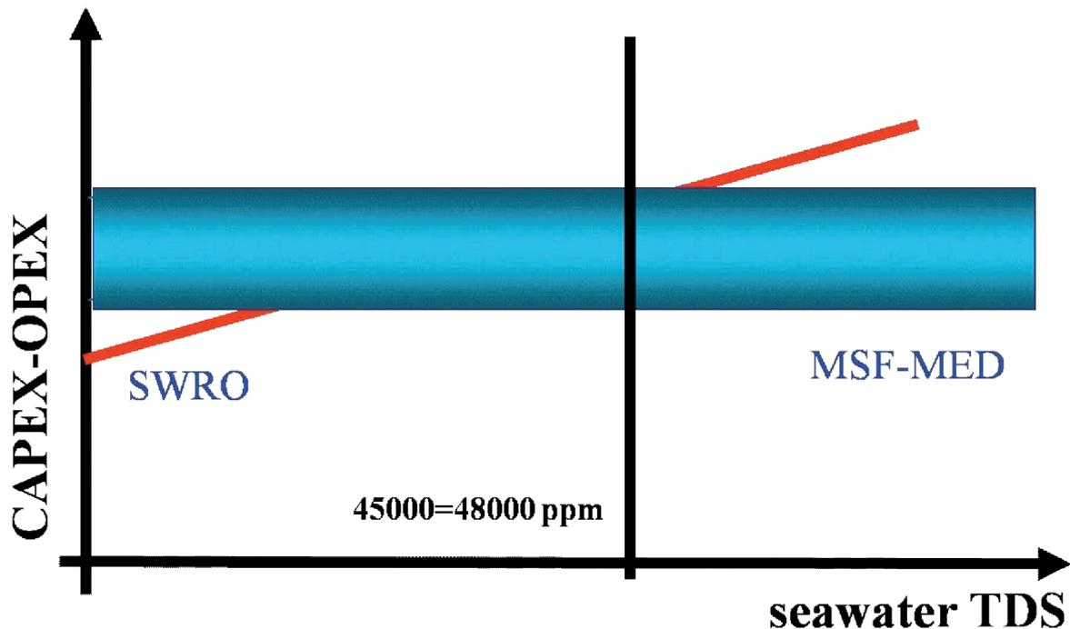
**Figure 6.6 typical cost trend CAPEX and OPEX versus TDS thermal and membrane technology**
