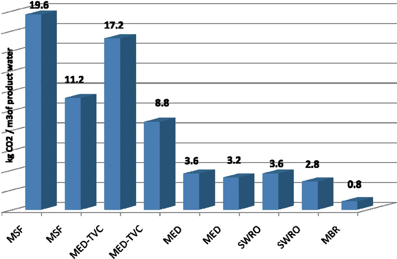
Figure 6.20: desalination technologies operating carbon footprint comparison
