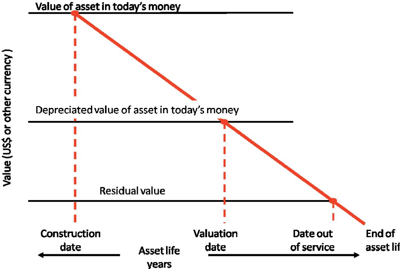
**Figure 9.2: equivalent assets value scheme**
