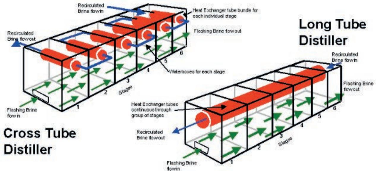
**Figure 5.2: MSF long tube and cross flow configuration**
