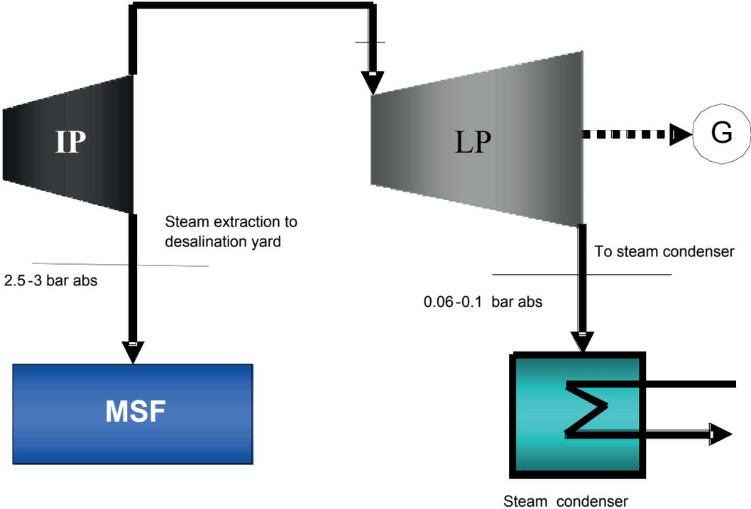
Fig. 6.8 condensing steam turbine feeding an MSF desalination system
