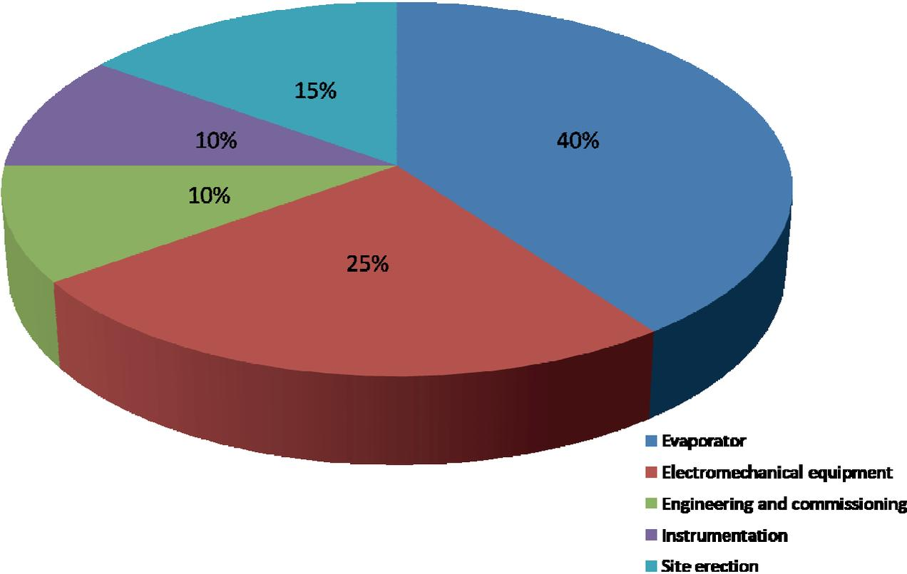
**Figure 14.4 : Thermal desalination plant cost component subdivision**
