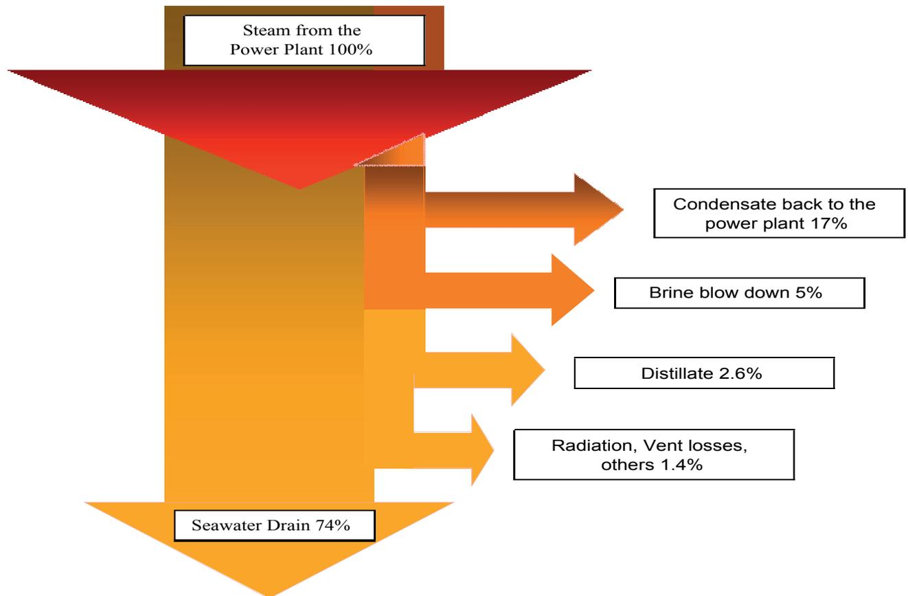
**Figure 6.4: Heat flow diagram thermal desalination plants**
