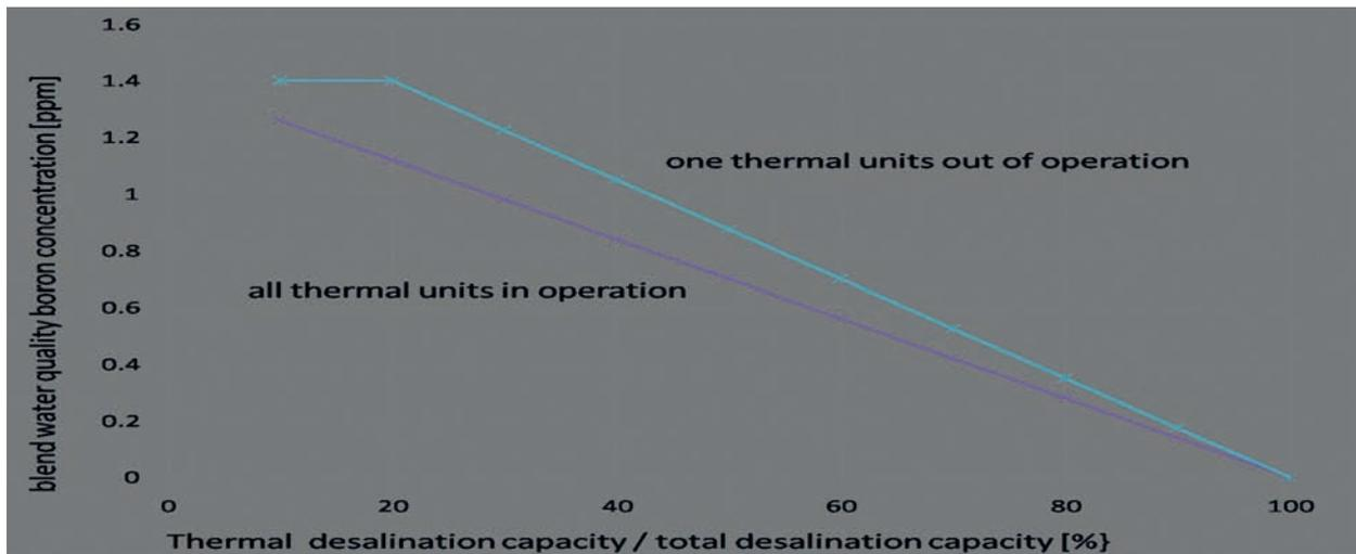
**Figure 5.9: product water quality against thermal / total product water capacity**
