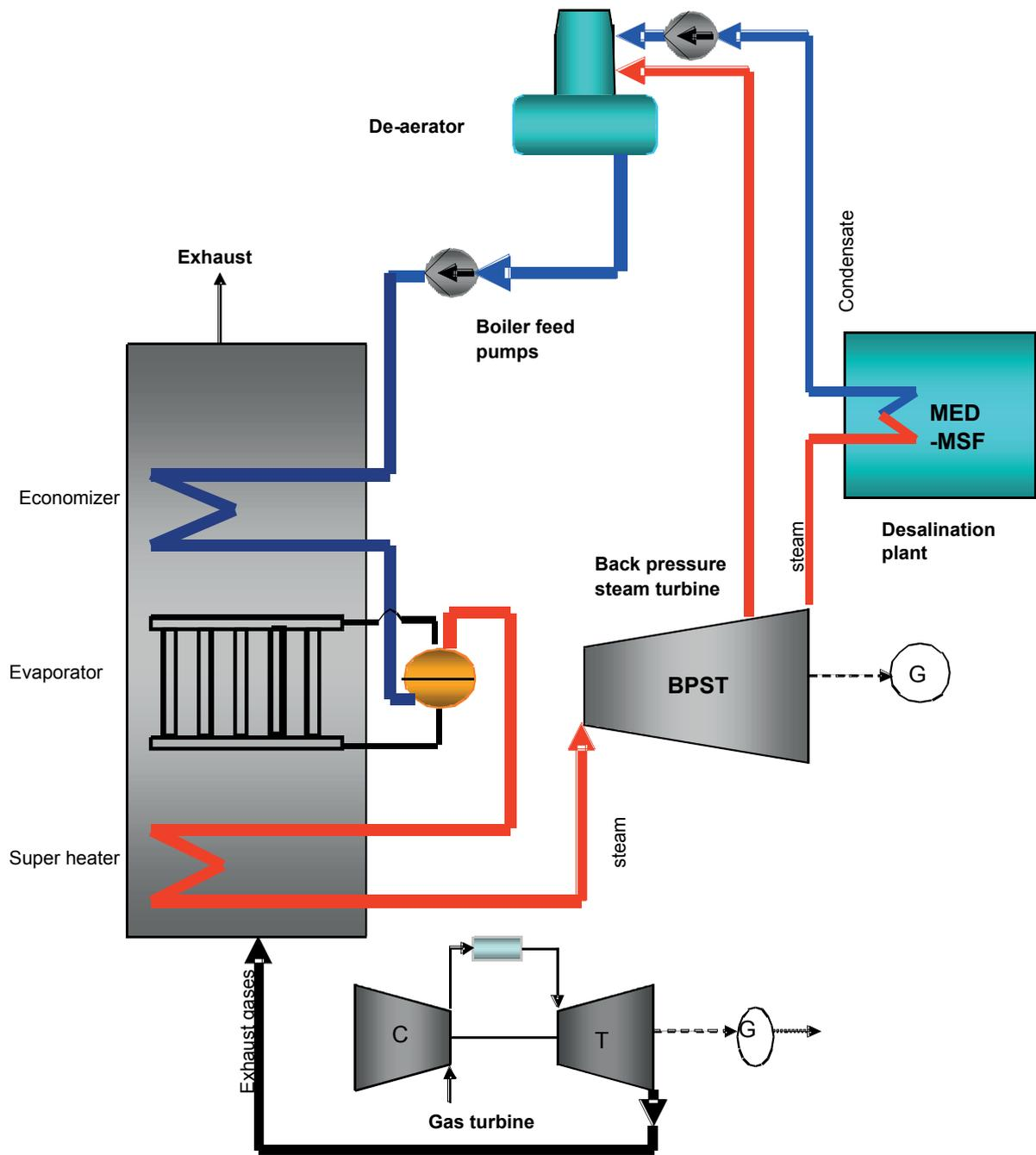
**Fig. 6.9 combined cycle with bottoming MSF-MED desalination system**
