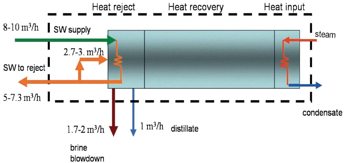
**Figure 6.3: seawater requirement MSF process typical flow sheet**
