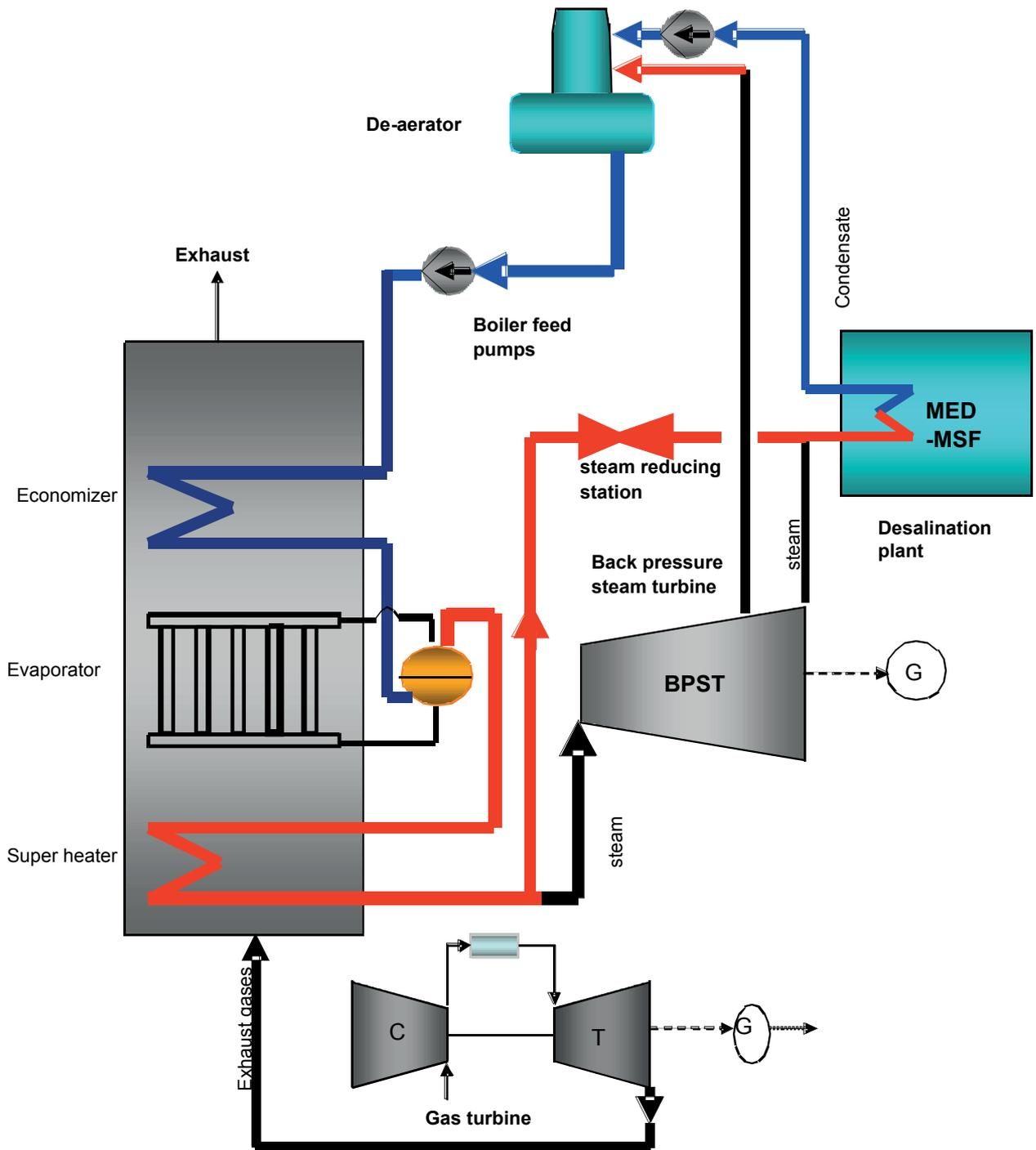
**Fig 6.12: Combined cycle with bottoming MSF-MED desalination system: winter operation**
