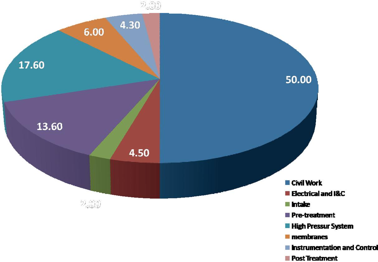
Figure 14.10 : SWRO cost breakdown : alternative case
