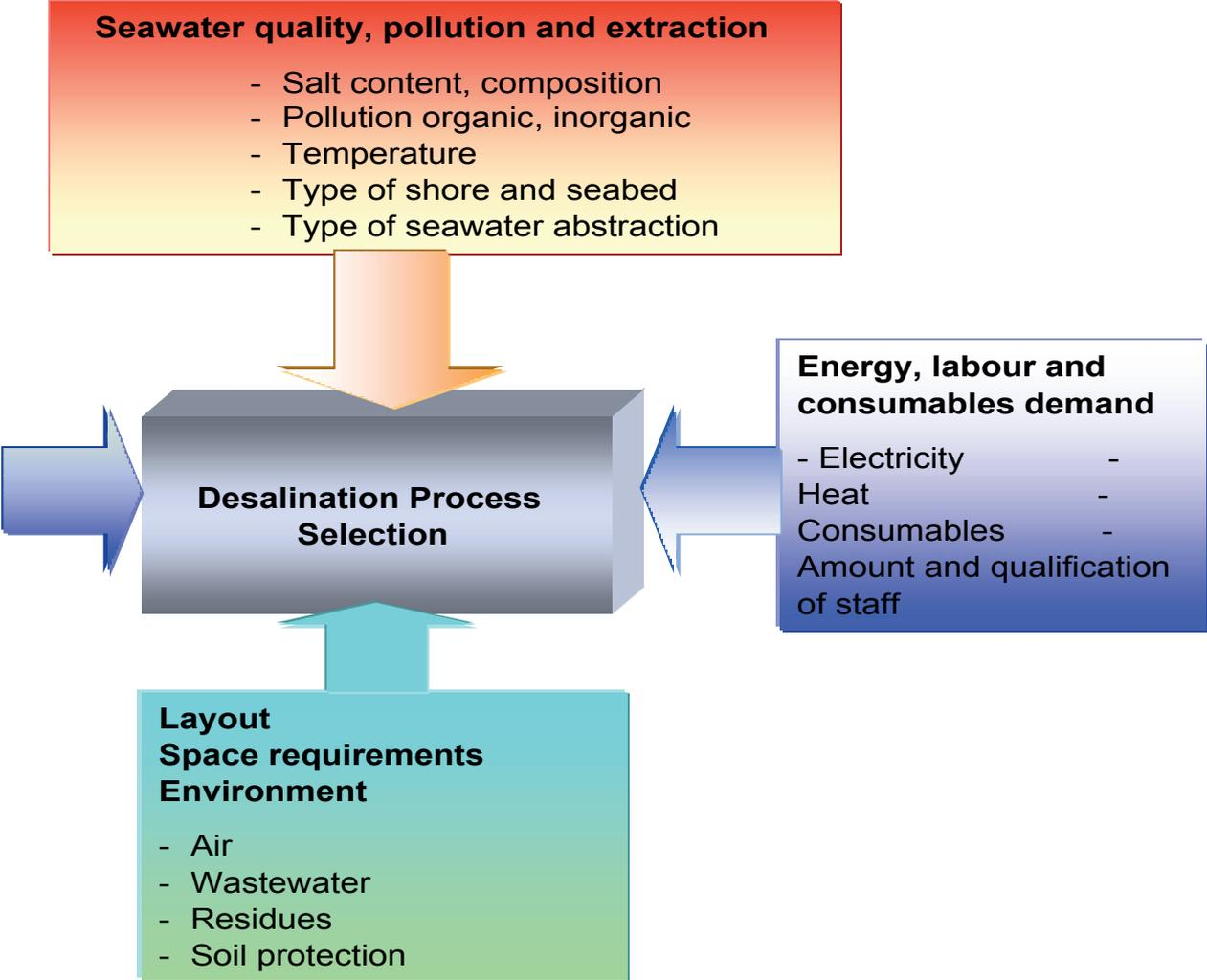
Figure 6.1: technology selection process – typical logic scheme
