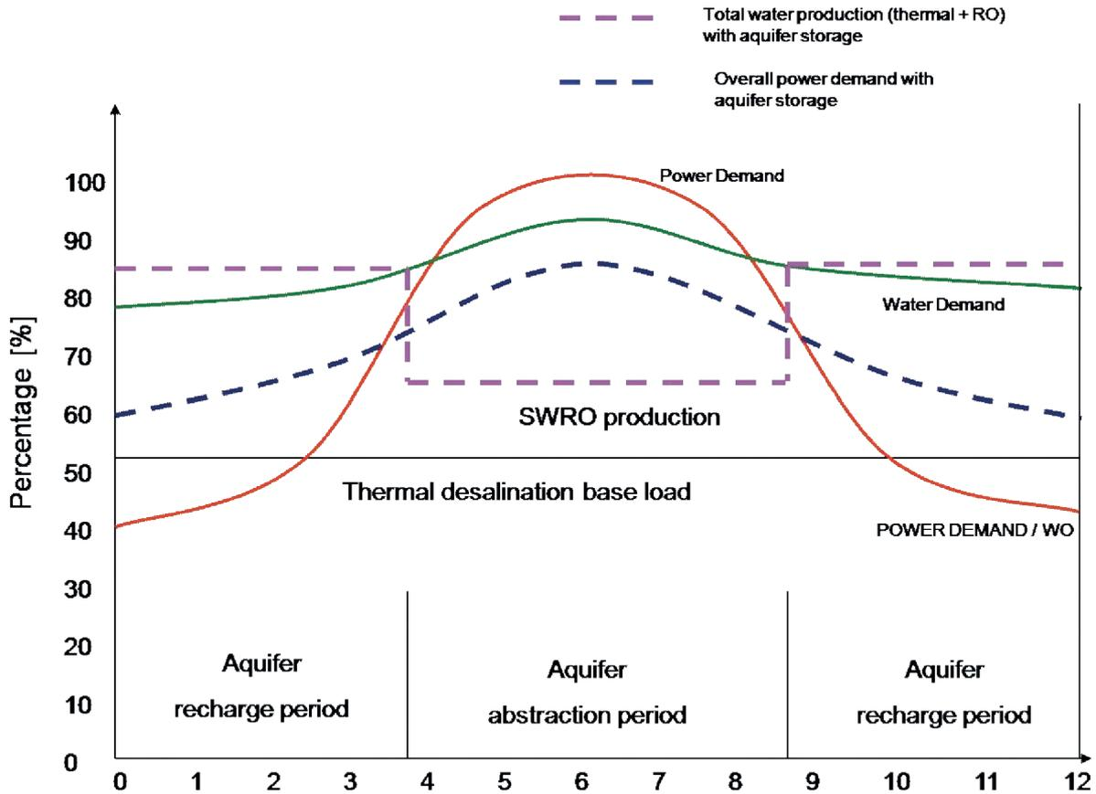
**Figure 5.6. Aquifer recharge and recovery (DASR) and peak load reduction effect**
