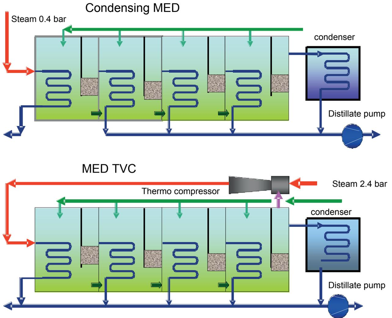
**Figure 5.3 condensing MED unit and MED-TVC schematic difference**
