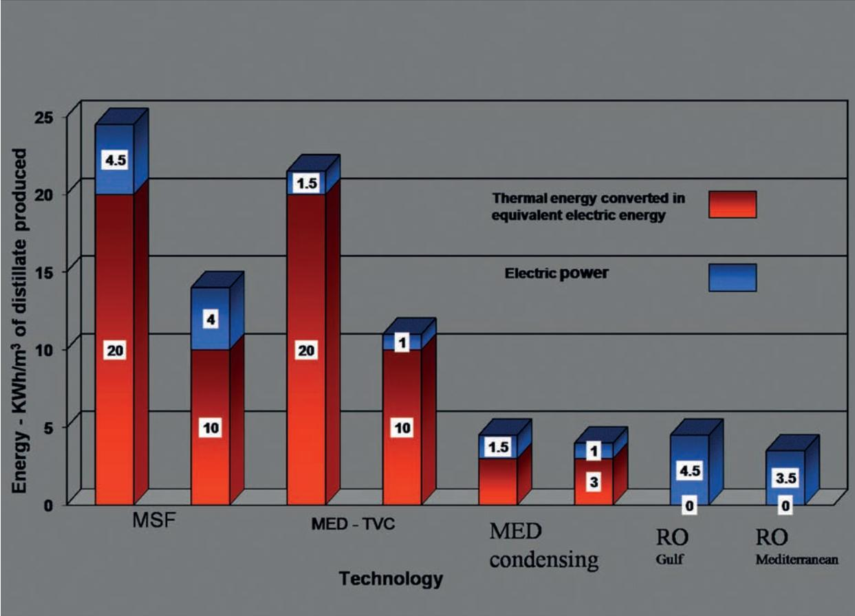
**Figure 6.10: Desalination technologies thermal and electric energy consumption** With reference to the values indicated in Fig 6.10 above it should be noted that, the difference in the energy requirements among the various technologies can become even larger if the steam for the thermal desalination plant is generated through auxiliary boilers or with large supplementary firing that decreases the plant heat rate.
