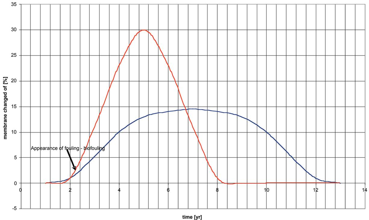
**Figure 7.5 Possible projected and actual membrane replacement rate as pre-treatment shortfall result**
