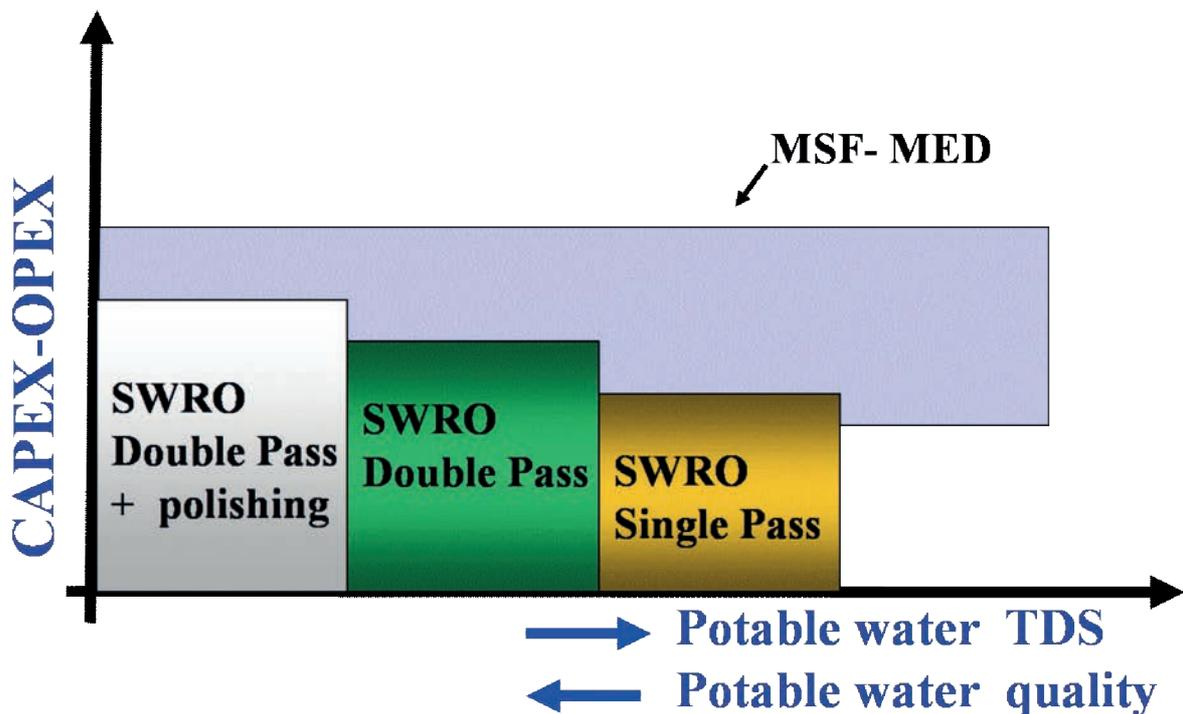
**Figure 6.7: CAPEX and OPEX at different potable water quality**
