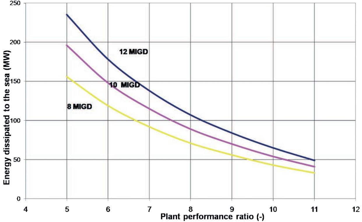
**Figure 6.5: energy dissipated with cooling water flow diagram thermal desalination plants**
