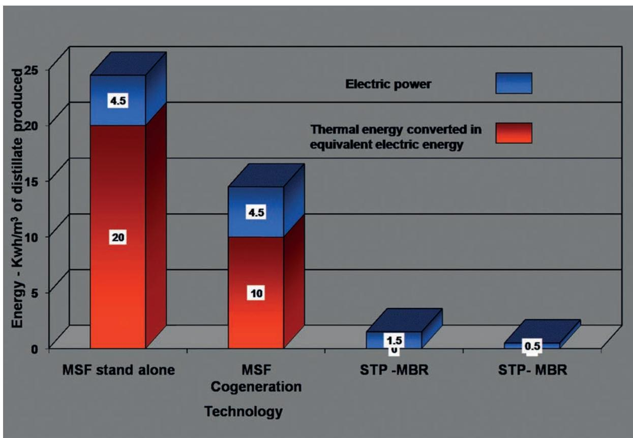
**Figure 6.15: thermal desalination and advanced water treatment energy footprint comparison**
