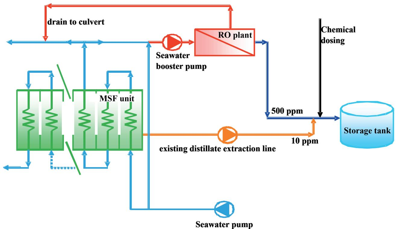
**Figure 5.8: Integrated hybrid system flow diagram**
