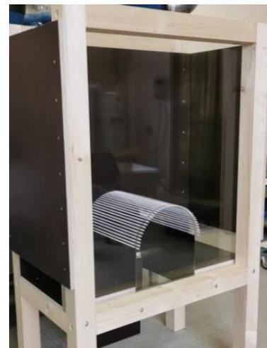
Figure 1. Model with a scale of 1:20 for experimental investigations (Pöchacker 2022)
