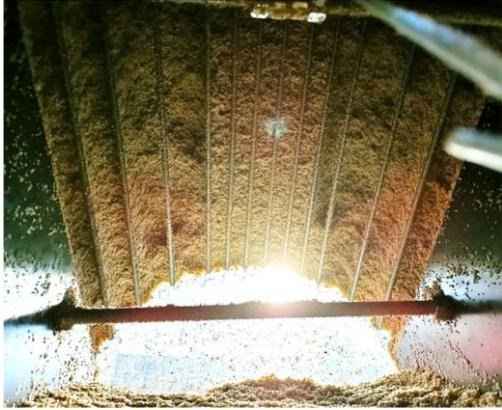
Figure 2. Arch formation between the pipes prior to failure, with  $\omega = 2\%$  and  $D_r = 0.98$ , (Pöchacker 2022)
