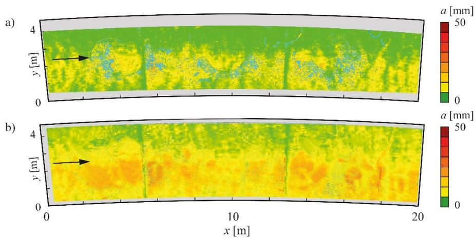
**Figure 6.** High-resolution abrasion maps of the 20 m long high-strength concrete test field C2 installed at test location 2 in Pfaffensprung SBT after (a) one and (b) two operational years (the grey colored areas could not be scanned due to ground water drainage installation).
