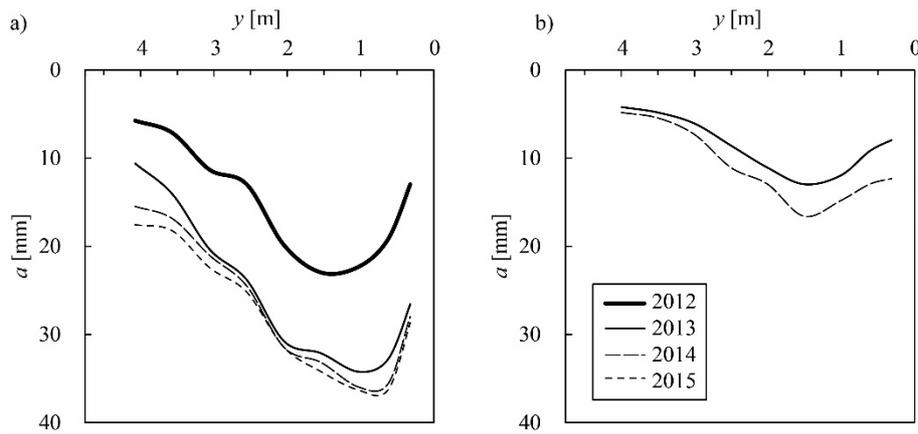
**Figure 9.** Super-elevated longitudinally averaged cross-sectional abrasion profiles of high-strength concrete test fields (a) C1 at test location 1 and (b) C2 at test location 2 installed at Pfaffensprung SBT for the years 2012 to 2015; view in flow direction.
