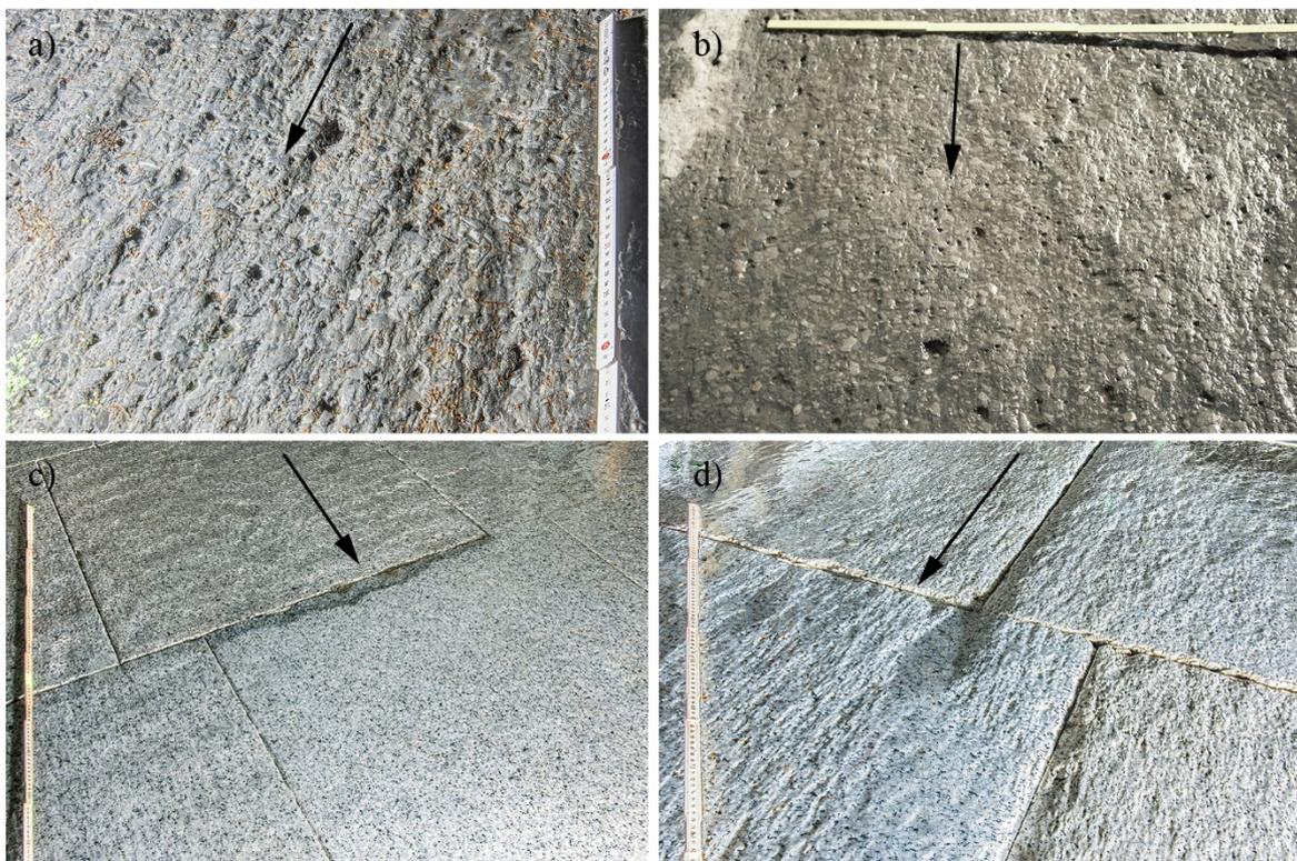
**Figure 4.** Close-up view of the abraded surface of the Pfaffensprung SBT: (a) high-strength concrete test field C1 after four operational years, (b) high-strength concrete test field C2 after two operational years, (c) granite test field G1 after four operational years showing abrasion concentration at upstream edges and (d) granite test field G1 after four operational years showing abrasion concentration along joints with downstream abrasion shadows.
