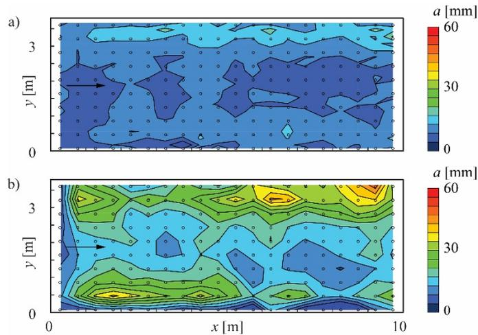
**Figure 11.** Abrasion depths of the silica fume concrete (SC) test field in Runcahez SBT in (a) 1999 after four years of operation and (b) 2014 after 19 years of operation (circles represent measurement points).
