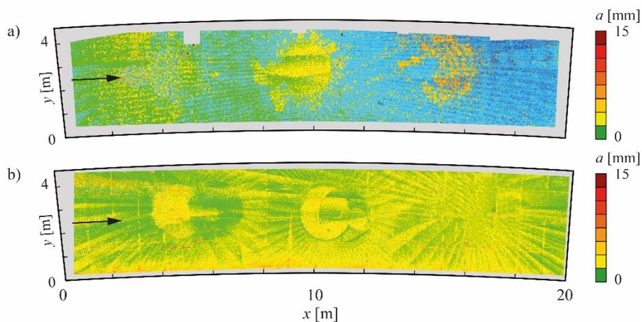
**Figure 8.** High-resolution abrasion maps of the 20 m long granite test field G2 installed at test location 2 in Pfaffensprung SBT after (a) one and (b) two operational years (blue colored points mark theoretically negative abrasion depths corresponding to detection uncertainty; grey areas could not be scanned due to ground water drainage installation).
