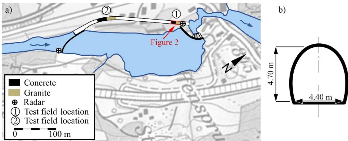
**Figure 1.** (a) Overview and (b) cross section of the Pfaffensprung SBT (position 46°42′49.8″ N 8°36′36.7″ E) with test field locations 1 and 2 and radar instrumentation for discharge monitoring, position of Figure 2 highlighted red.
