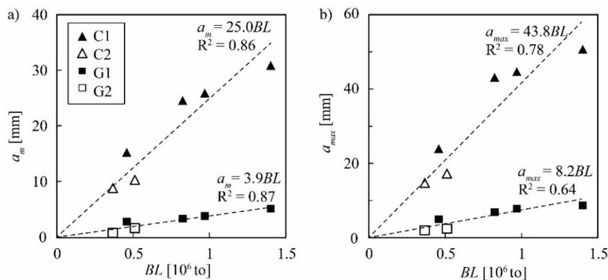
**Figure 10.** (a) Mean and (b) maximum cumulative abrasion depths as a function of cumulative bedload mass at Pfaffensprung SBT for high-strength concrete test fields C1 and C2 and granite test fields G1 and G2 for the years 2012 to 2015.
