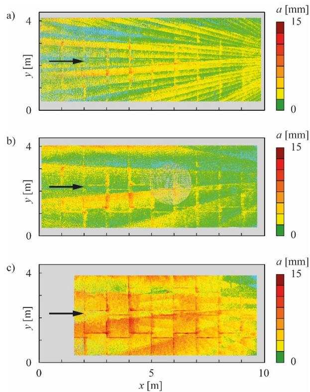
**Figure 7.** High-resolution abrasion maps of the 10 m long granite test field G1 installed at test location 1 in Pfaffensprung SBT after (a) one, (b) two and (c) four operational years (blue colored points mark theoretically negative abrasion depths corresponding to detection uncertainty; grey colored areas could not be scanned due to ground water drainage installation).
