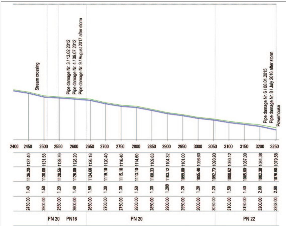
Fig. 1. Detail from drawing depicting pipe damage incidents (prepared by the operating company).
