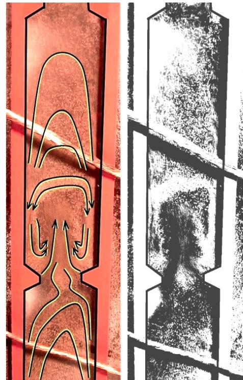
**Fig. 10: Particle movement above constriction**
