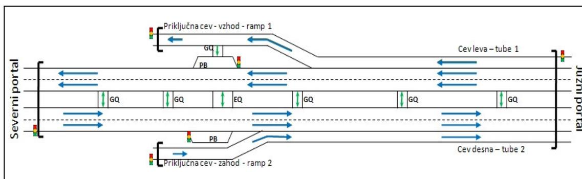
Picture 8: System of tunnel Šentvid with emergency exits
