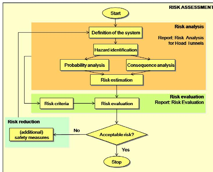
Picture 2: Flowchart of the procedure for risk assessment (PIARC 2008, Risk Analysis for Road Tunnels).
