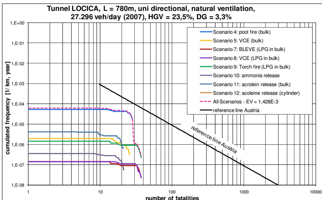
Picture 7: Resulting F/N-curves for DG risk in comparison to the reference line – current situation (2007)
