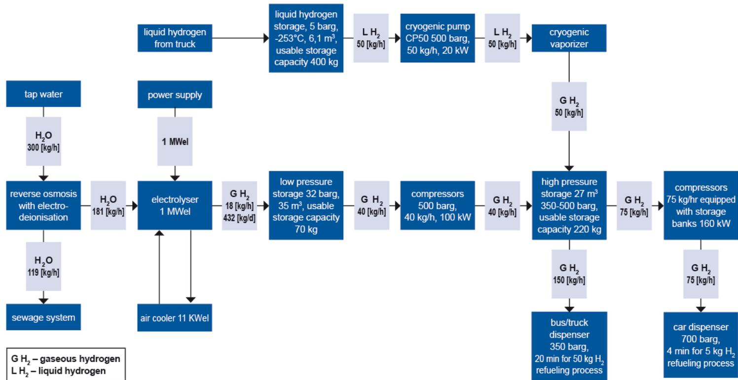
Figure 1 Technological train together with main equipment arrangement
