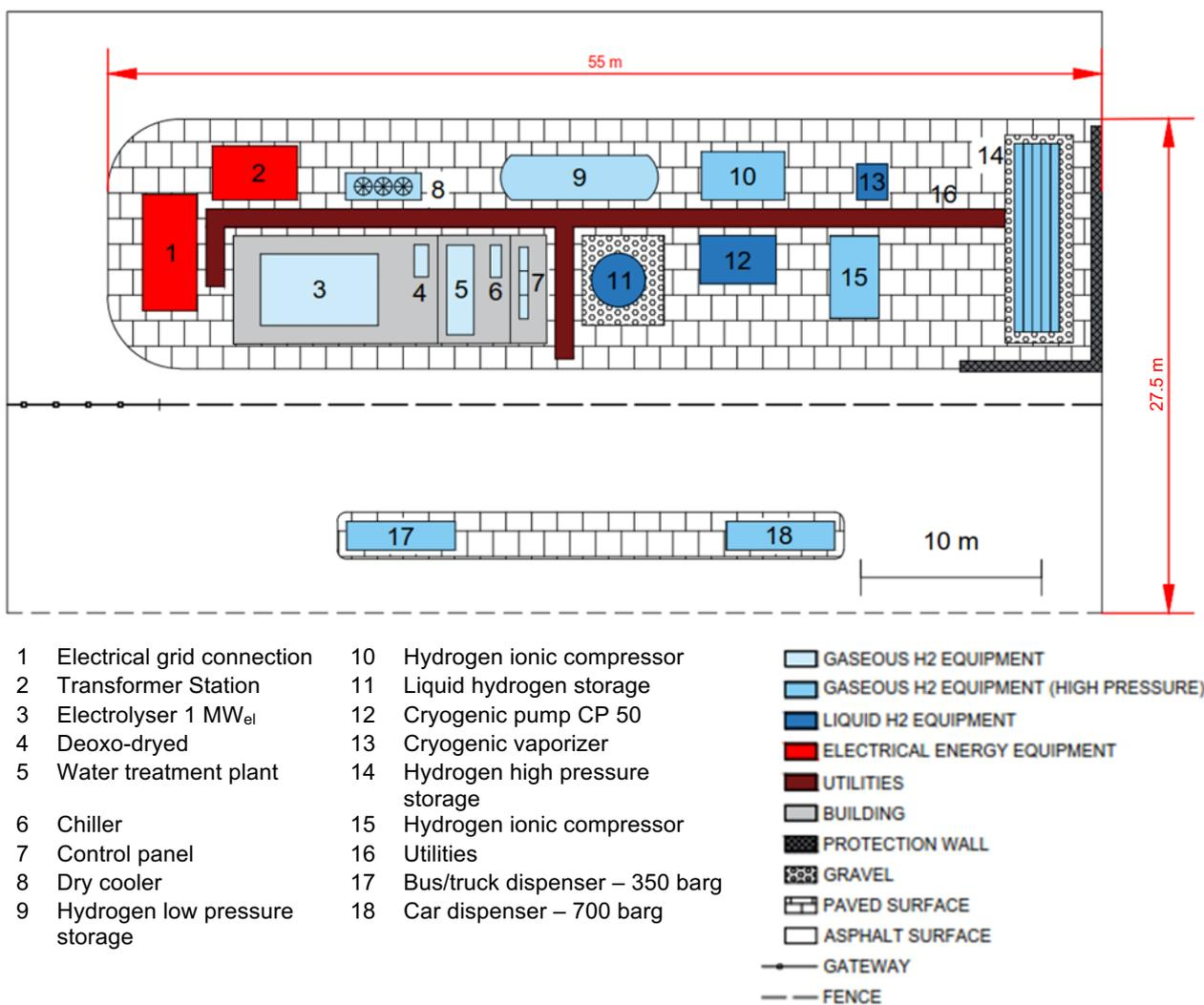
**Figure 2** Layout of a fuelling station with electrolyser
