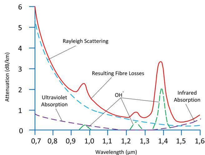
Figure 2. Causes of attenuation in optical fibres.
