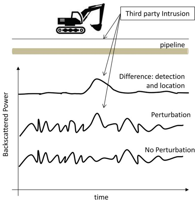
Figure 5. Intrusion detection through DAS.
