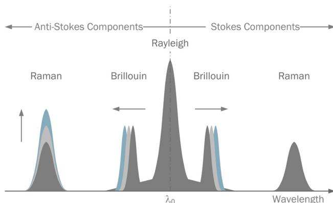
Figure 3. Frequency response of backscattering light.
