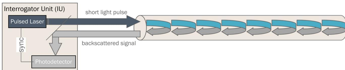
Figure 6. A DAS Interrogator Unit receiving backscattered signals from the fibre.
