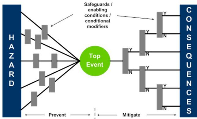
Figure 4. Example of a typical bowtie diagram.
